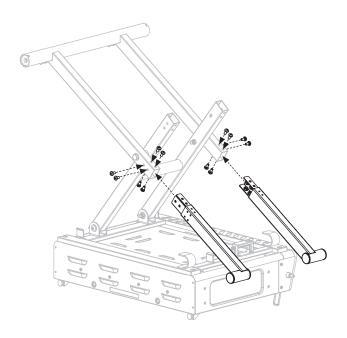
$\underline{\textbf{STEP 04}}$  Use twelve (12) M6x12 screws (**a**) to install the lower leg assembly onto the fixed leg assembly.
