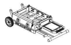
**STEP 10** Lift the side shelf handle and, while putting weight on the fixed leg assembly crossbar, pull the griddle up and toward you until the top of the wheeled leg assembly aligns with the C clamps.
