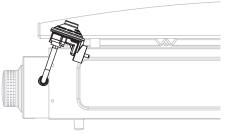
**PLEASE NOTE:** The gas regulator is intended be used at an angle towards the rear of the griddle as shown above.
