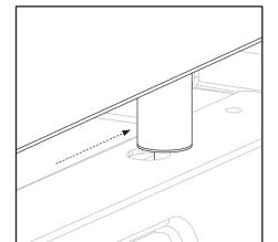
Ensure that the front pins are fully seated in the holes, then push the griddle top forward to lock the griddle in place.
