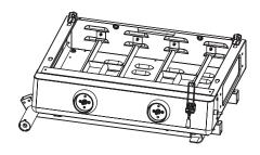
**STEP 02** Turn the griddle body upside down, and pull the locking pin to unlock the legs.
