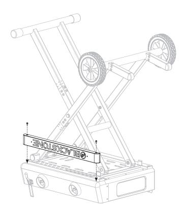
**STEP 08** Use four (4) M6x12 screws (**a**) to install the side shelf to the right side of the griddle body.
