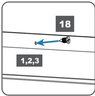
Secure the pre-assembled screen frame (1) and (7) with screws (18) on the horizontal direction, and screw (14) in the parallel directions.
