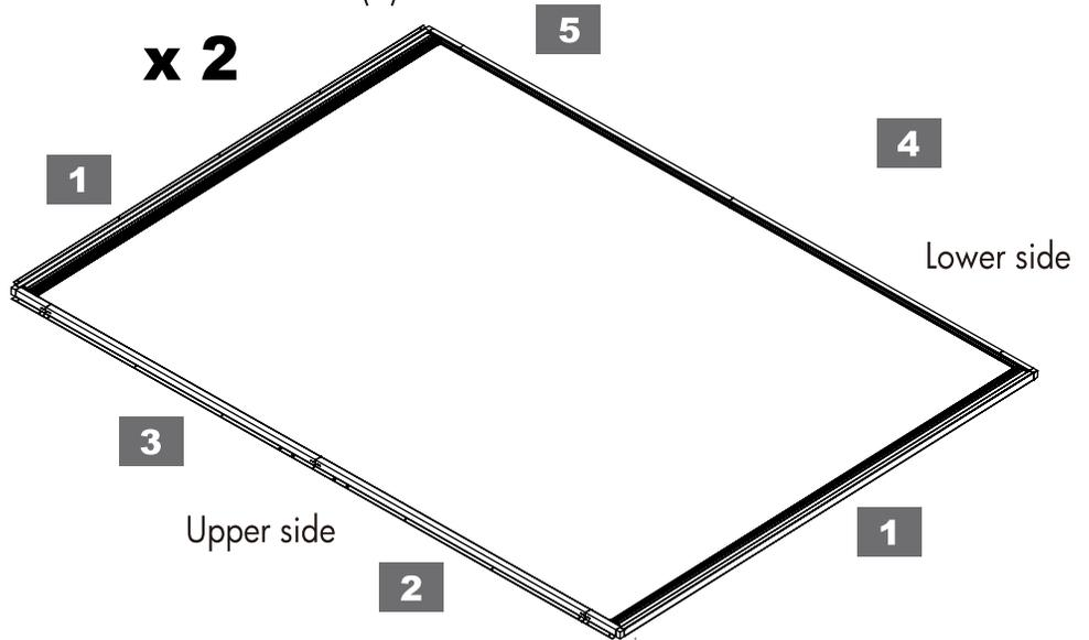
Attach upper frame B (3) to screen (1), upper frame A (2) to upper frame B (3) and the other end to screen (1) with screw (13).
