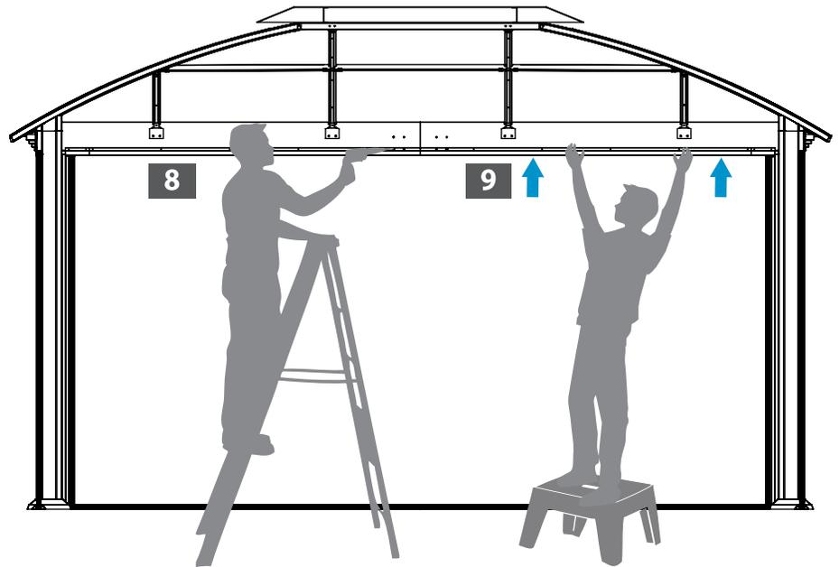
It is **REQUIRED** to lift up the upper side of screen and rail at the same time before using the screws to secure screen (1) to the rail as shown.
