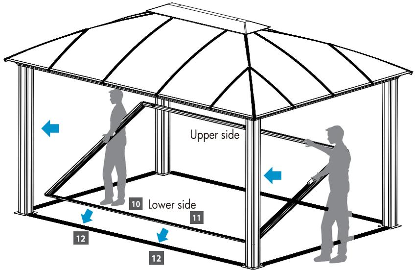
Attach upper side of screen (7) to the rail, using the screws you have just removed from the middle of the rails to the same position to secure screen (7).
