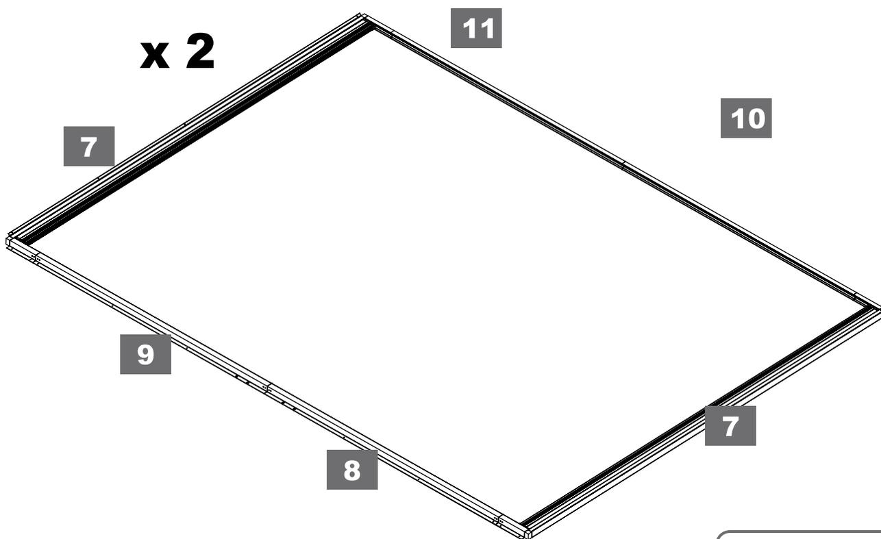
Attach upper frame D (9) to screen (7), upper frame C (8) to upper frame D (9) and the other end to screen (7) with screw (13).
