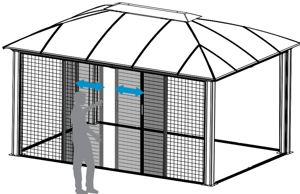
Test the screen by pulling to left and right a couple of times, make sure the screen is functional.
