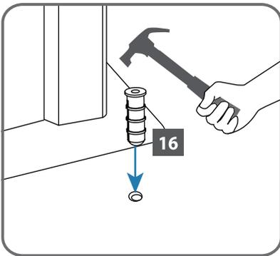
Insert part (16) into the hole by a hamer. Place lower frame C (6) and F (12) to the same position of step 2.A, and fix it with screws (15), washer (17) into the pre-drilling holes.
