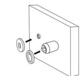
8. Once installation is complete, turn on the main water supply. Use the provided tool to remove the aerator from the spout. Turn the water on to allow any dust or loose sediment to clear the system. Allow the water to flow through the spout for approximately 60 seconds, and verify that hot and cold water are running properly. Reattach the aerator once testing is complete.
