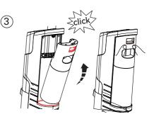
Align the bottom of the clean water tank with the grooves and push the tank until it "clicks" into place.
