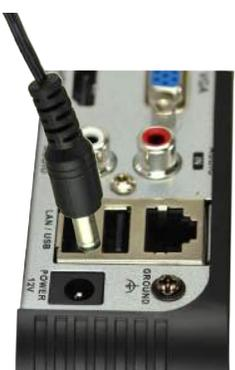
**J** Connect the DVR power adapter to the Power Input on the rear of the DVR.
