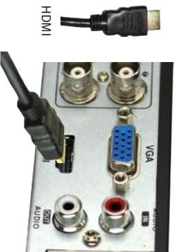
**A** Plug one end of the included HDMI cable into the HDMI port on the back of the DVR.
