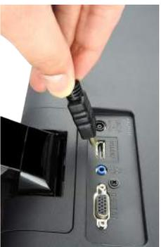
**B** Plug the other end of the HDMI cable into the back of your TV or monitor.
