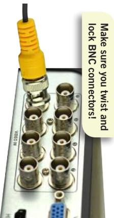
**F** Connect the BNC connector of the video/power cable labeled **TO DVR ONLY** to an open video input on the DVR.
