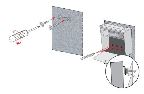
Using a masonry style drill bit(not provided), drill the bottom three pilot holes approximately 2 inches deep into the wall material. Now hang the Townhouse from the mounting bracket and secure to bottom using the three 21/4" screws provided. Be sure to put some weather resistant caulk into the holes..lf your wall is a thick brick, stucco or concrete you will may need masonry screws or anchors for attachment, consult a contractor if necessary.
