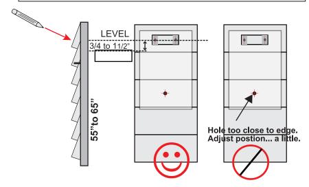
Using a 1/8" drill bit, drill the top two pilot holes approximately 2 inches deep into the the wall material. Attach the mounting bracket using the two 21/4" screws provided. Be sure to put some water resistant caulk into the holes. Now hang the Townhouse from the bracket as shown and mark the bottom three holes with a pencil.
