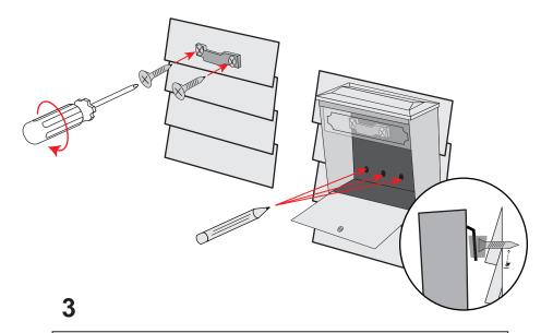
Using a 1/8" drill bit, drill the bottom three pilot holes approximately 2 inches deep into the wall material. Now hangy our Townhouse from the the mounting bracket. If there is a large gap between the Townhouse and the wall insert a bushing on the screw. Insert some water resistant caulk into the hole and secure to bottom using the remaining three 21/4" screws provided.
