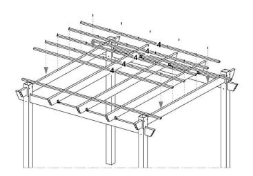
Using 1¼" painted screws, fasten remaining top cross rails (part 4) to upper supports.
