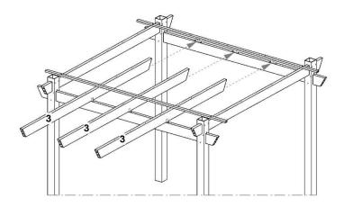
Slide three remaining upper support rails (part 3) through upper support brackets, underneath top rails.
