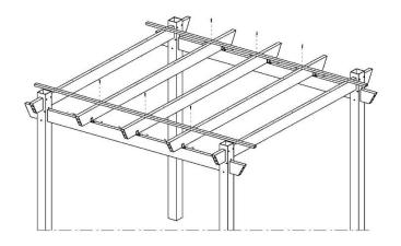
7 Using 1¼" painted screws, fasten top cross rails to upper supports.
