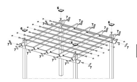
Using included Super Glue, glue post caps (part 6) to top of posts. Glue support end caps (part 7) to ends of upper and lower supports. Glue % x 1½" end caps to ends of top cross rails.
