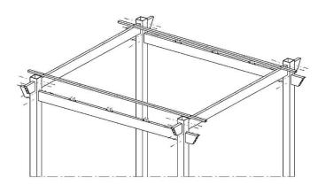
Using 2" painted screws, screw together all posts and supports.
