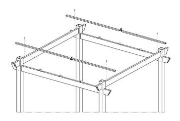
Lay two top cross rails (part 4) onto upper supports. To set width of pergola, line up outer most holes of top rails with outer most pilot holes of upper supports. Using 1½" painted screws, fasten top rails to upper supports.
