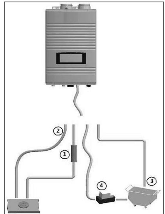
**Figure 12 – Condensate Detail**
