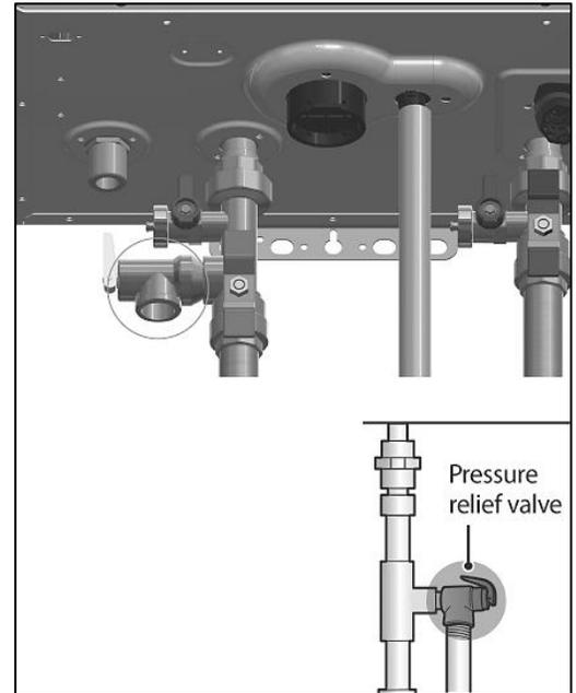
**Figure 19 – Relief Valve Details**
