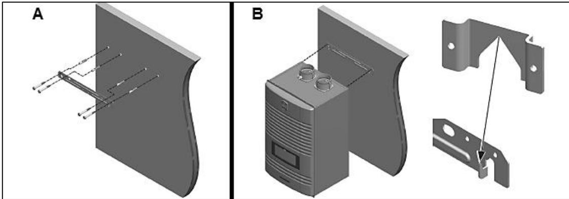
Figure 4 – Wall Mounting the Water Heater
