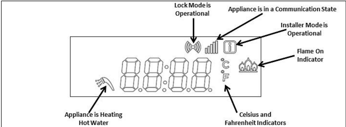
Figure 25 – LCD Display Detail
