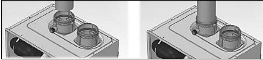
Figure 6 – Correct Installation into the Water heater Collar
