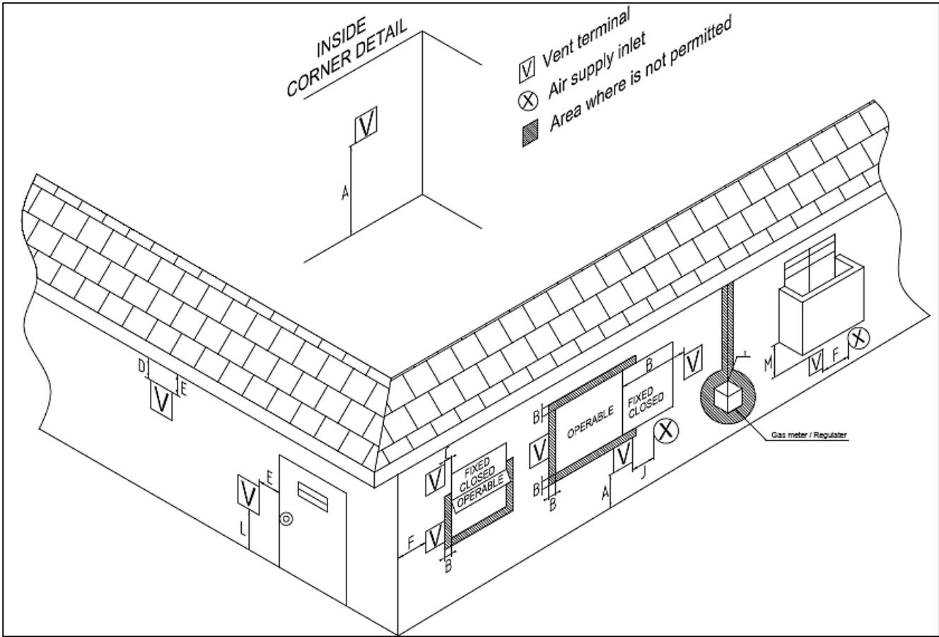
Figure 5 – Vent Termination Detail
