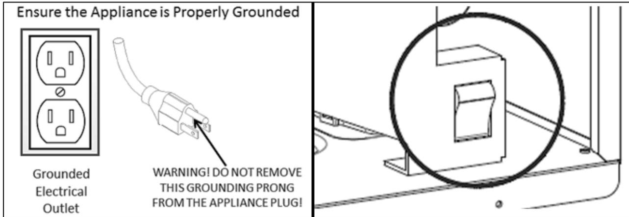
**Figure 20 – Proper Grounding – Internal Manual Power Switch**
