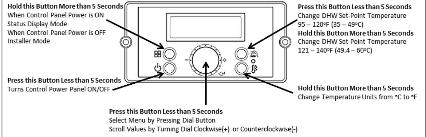
Figure 24 – Water heater Control Panel Detail
