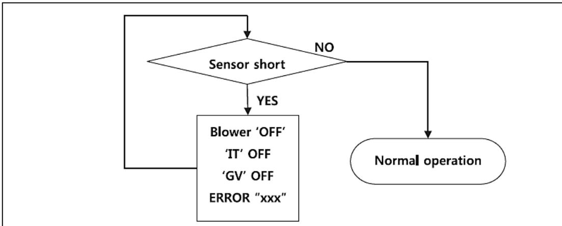
Figure 34 – Inlet / DHW / Operating Temperature Sensors Error Analysis Tree
