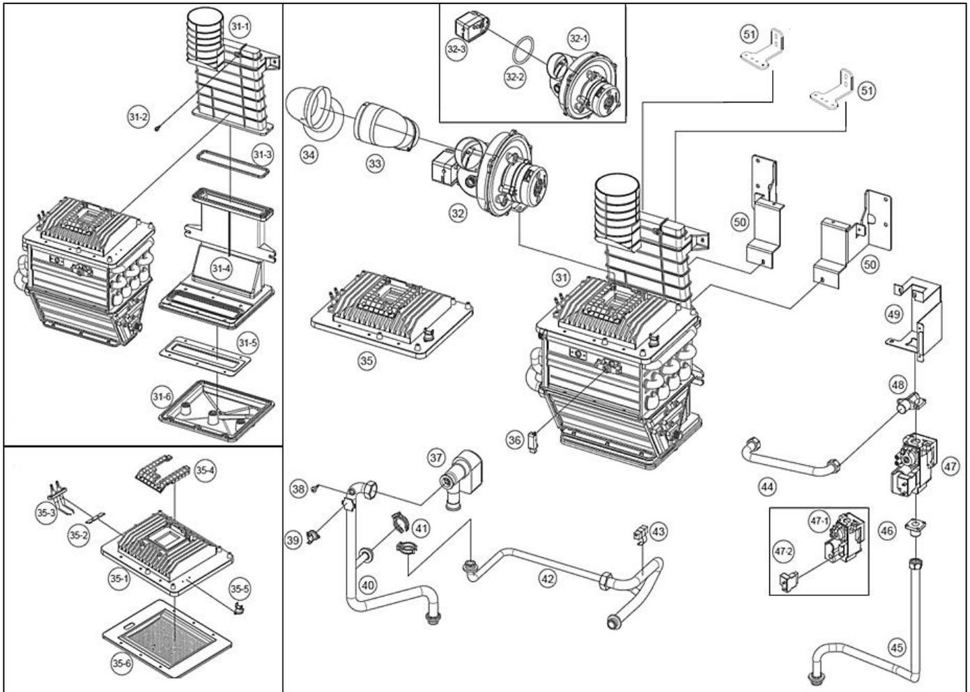
Figure 40 – Heat Exchanger Replacement Parts
