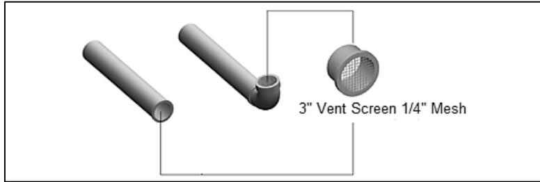
**Figure 11 – Screen Installation - NOTE: Vent termination elbow is meant to be installed open end facing the ground. Orientation in Figure 11 is meant to demonstrate proper Vent Screen installation ONLY.**
