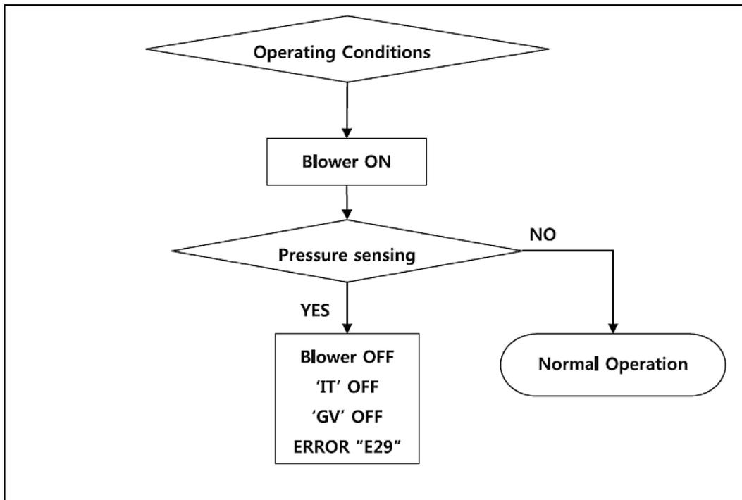
Figure 33 – Air Pressure Switch Analysis Tree
