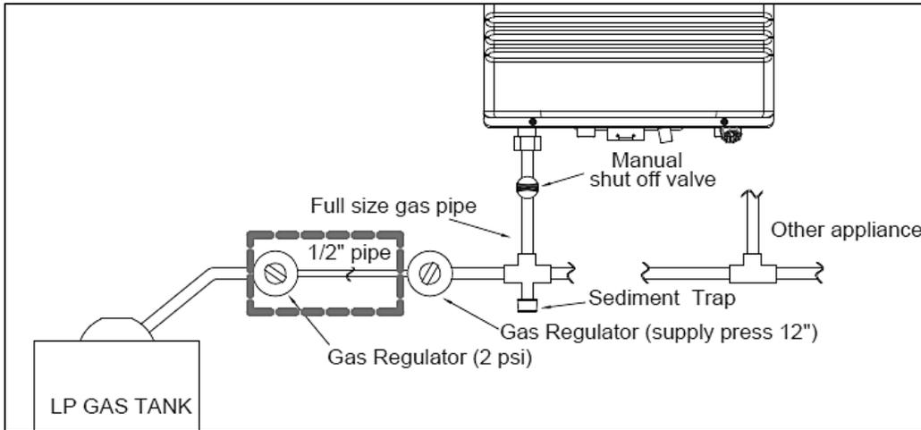
Figure 15 – LP Gas Piping Installation – NOTE: Capacity to be Not Less than Total Capacity of Connected Appliances
