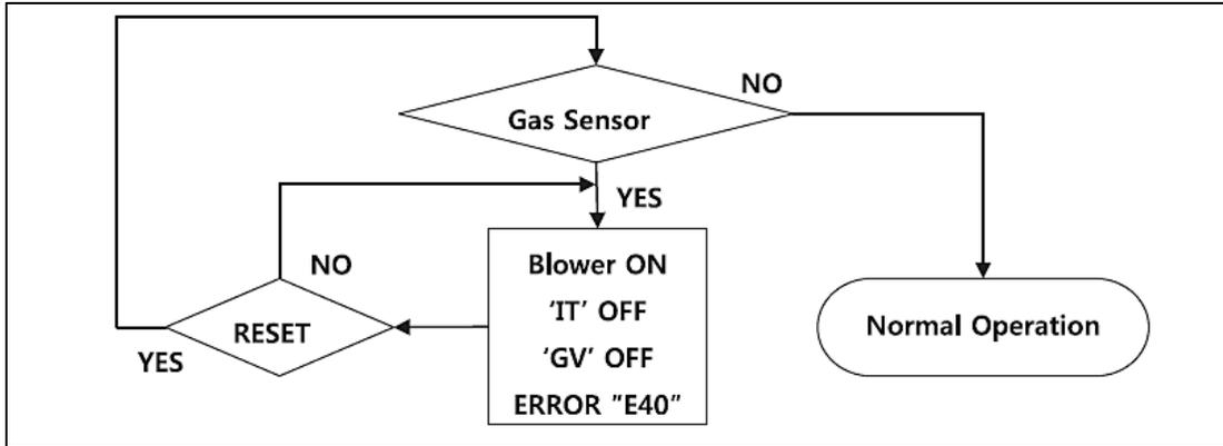
Figure 32 – Gas Detection Error Analysis Tree
