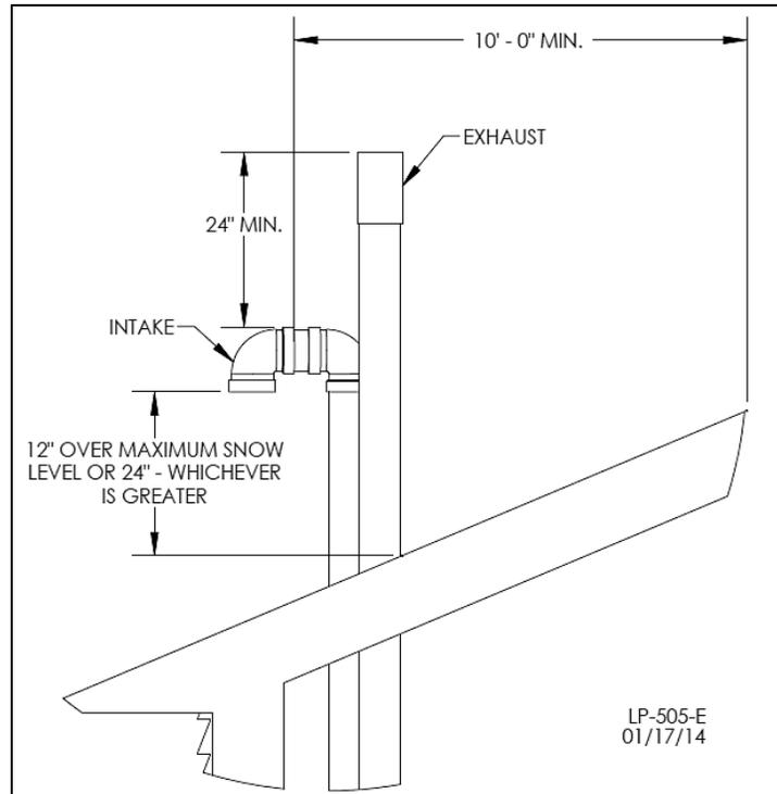
Figure 9 – Direct Vent, Vertical Termination
