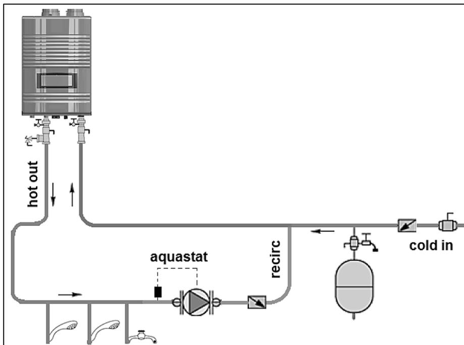
Figure 18 – Piping with Recirculation
