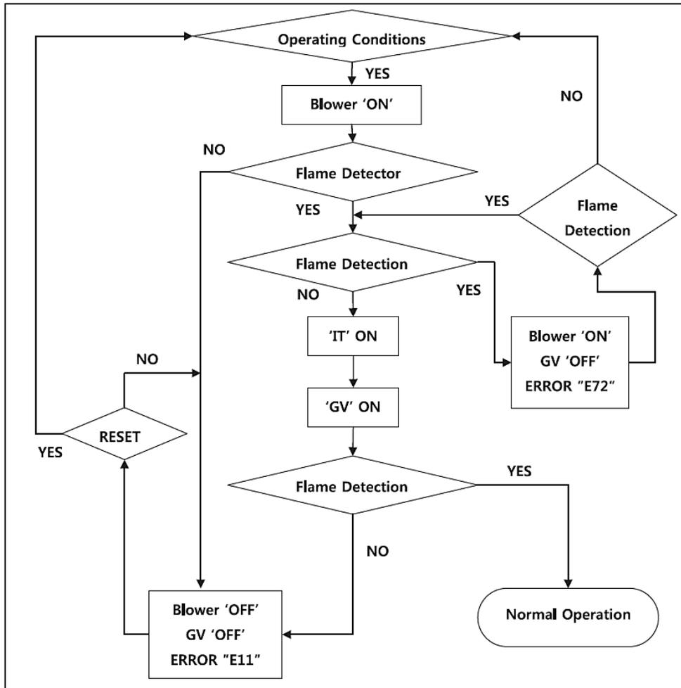
Figure 31 – Flame Detection Error Analysis Tree
