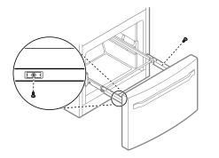
Grip both sides of the drawer and pull it up to remove it from the rails.
