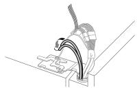
5 Hold the water supply connection and gently push in the collet ④ to connect the water supply lines as shown. Insert the tube at least 5/8 inch (15 mm) into the connector. Insert the clip on the joint to fasten the tubes in place.
