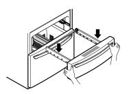
**2** Pull the drawer open to full extension. Lower the basket onto the rails.
