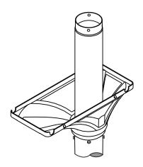
3 Attach the mounting plate to the post using the 4 small hex bolts, nuts and 8 small washers.
