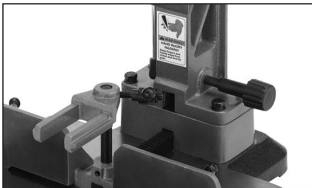
Figure 16. Extension block installed.
