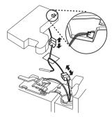
Rotate hinge lever counterclockwise. Lift the top hinge free of the hinge lever latch.
