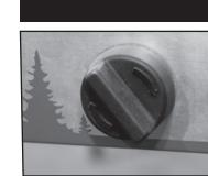
Fully open LP bottle valve. Turn valve to medium position. Allow gas to flow to burner. Immediately turn rotary ignitor. The ignitor should spark and light the burner. If ignition does not occur in 5 seconds, turn the burner control(s) off, wait 5 minutes, and repeat the lighting procedures.
