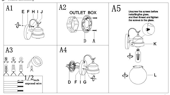
Step A1: Thread screw (J) through the plastic washer (I), then fix the flat iron bar (H) to the back plate (F) and lock with nut (E).
