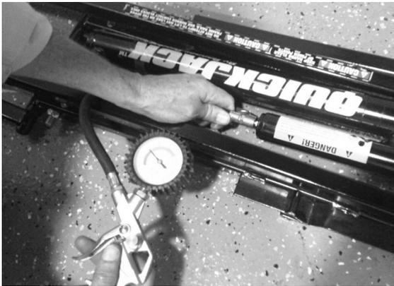
3. When the pressure is between 40 and 50 psi / 2.75 to 3.4 BAR, remove the pump or air compressor.
