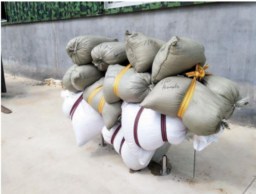
Photo 1: Panel loaded vertically with 2,520 pounds.
