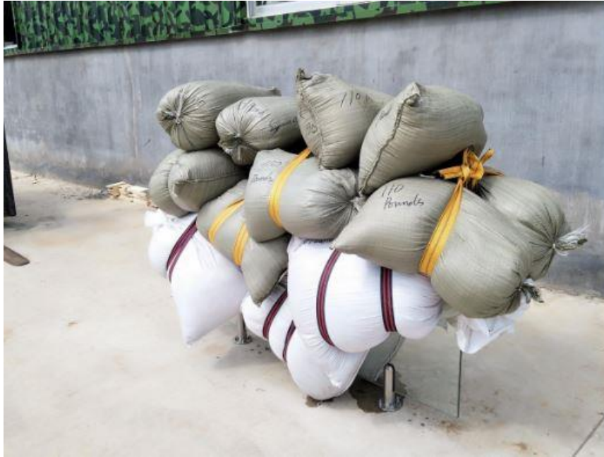
Photo 1: Panel loaded vertically with 2,520 pounds.
