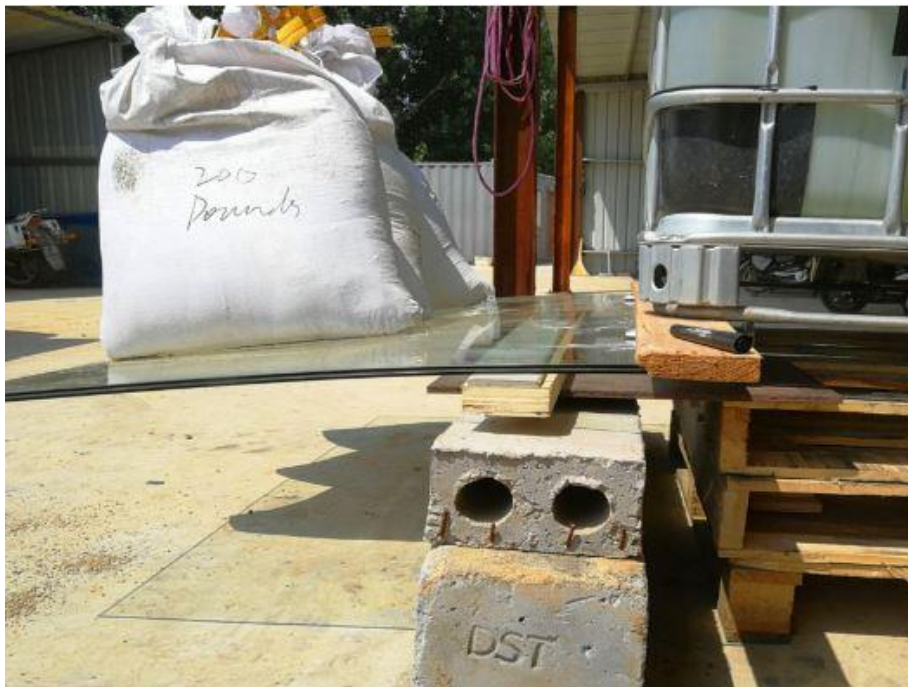
Photo 2: Loading of panel with sandbags, simulating horizontal force
