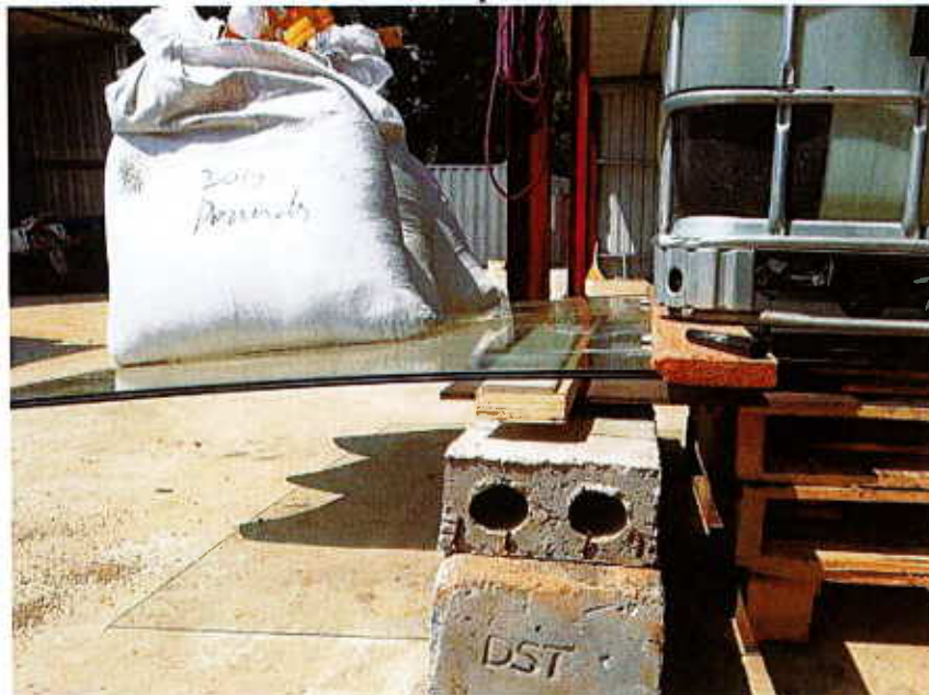
Diagram 1: Test rig lying on its side, looking from above, showing panel supported at 28 inches and at bottom of panel
