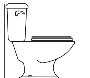
Mat can be installed under tile to within 4"-6" from the wax ring, and can slightly underlay the foot of the toilet if need be (approximately 20" from wall).
