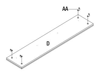
b) Semi-fix L shaped bracket(AA) with short hexagon socket screw(BB)  $\square$  c) Align shelf support(E) to holes on fixed shelf(D)
