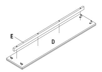
d) Tightening shelf support(E) with cross round head screw(FF)
