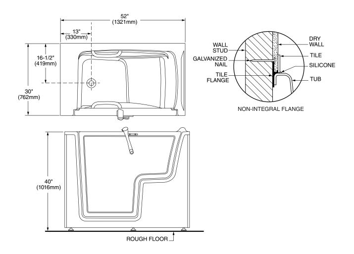
Tubs installed in an alcove installation require a raised flange to prevent water from seeping past the tub and into the wall. Tubs without a raised flange shall be installed with a tile flange kit such as model: 9FLNG or a similar type. The flange kit is a long plastic strip that fits onto the rim of the tub to provide the leak protection needed.
