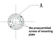
3) Put the back plate (C)onto the screws of mounting plate (A)and secure with ball nuts (K)
