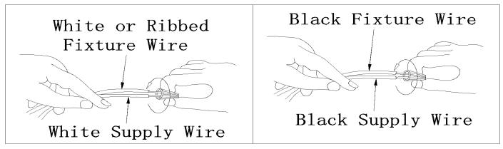
Twist plastic wire connector until wires are tightly joined together, wrap each connector with approved electrical tape for more secure connection .  $\qquad \qquad B \qquad A$
