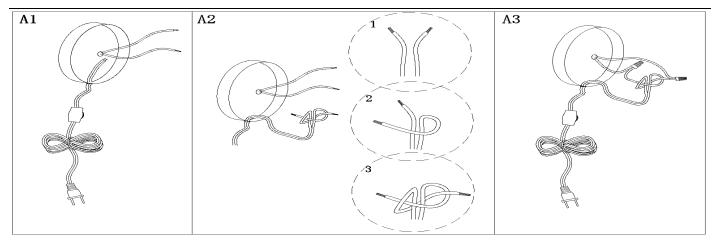
Step A1: Pass the power cord through the hole in back plate
