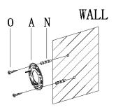
Note :the preassembled screws of mounting plate(A)should be horizontal direction after the mounting plate mounted. If not, rotate carefully the mounting plate side to side until the angle is achieved, tighten the wood screws(o).
