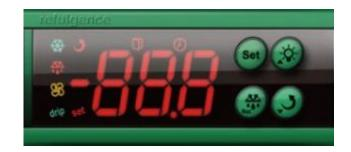
When the parameter item is selected, press **Set** key to enter to the setting of the current item, press or to modify the value, and then press **Set** key to return to menu. Under the status of parameter setting, press key or no key operation within 30s, it will exit from parameter setting and automatically save the current parameter value.
