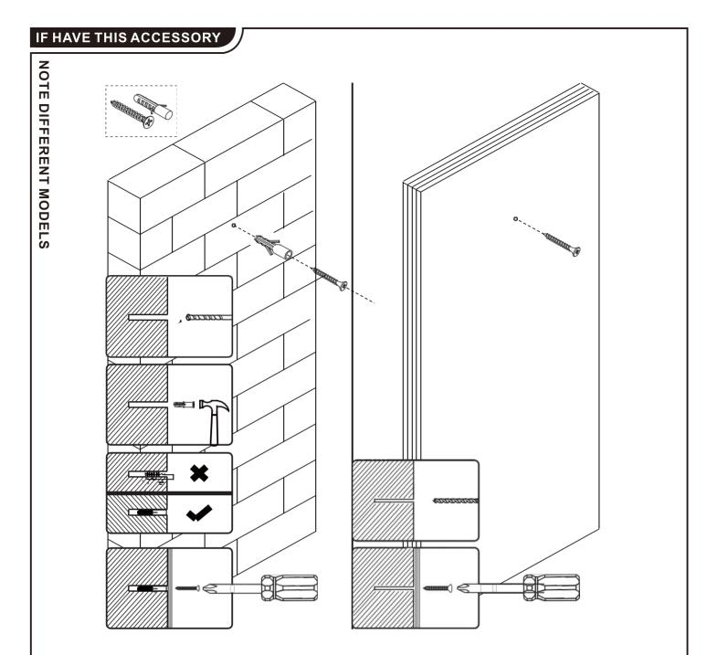
If it is a solid wall, please use expansion and self-tapping screws, if it is a wooden wall, only use self-tapping screws, please do not overtighten the screws.
