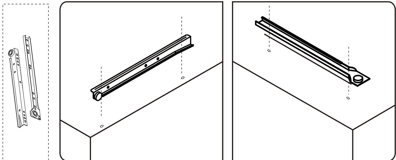
Please find the exact hole for installation, otherwise it will be misaligned. The screws on the drawer slide must be leveled, otherwise it will affect the smoothness of the drawer.
