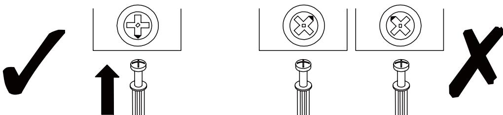
**CAMLOCK:** When fitting cam lock, ensure starting position is correct before you insert connecting quickfit.
