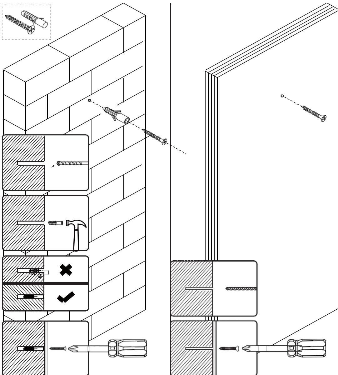
If it is a solid wall, please use expansion and self-tapping screws, if it is a wooden wall, only use self-tapping screws, please do not overtighten the screws.
