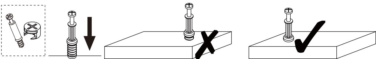
**QUICKFIT:** Tighten quickfit until shoulder is flush with panel. Do not overtighten or undertighten.
