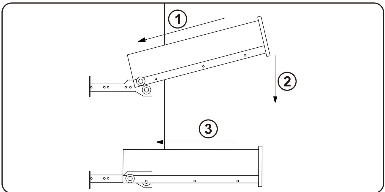
Be careful to push in the board when the both sides slide way been aligned.
