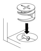
Qucikfit head should be in the centre of the cam lockwhen the two panels are joined. Cam lock should be inserted before quickfit.
