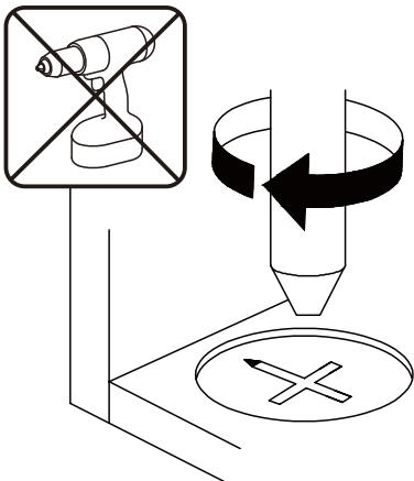
Turn cam lock clockwise to tighten.
