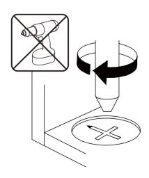
Turn cam lock clockwise to tighten.
