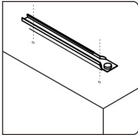
Please find the exact hole for installation, otherwise it will be misaligned. The screws on the drawer slide must be leveled, otherwise it will affect the smoothness of the drawer.
