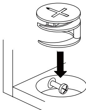
Quicikfit head should be in the centre of the cam lockwhen the two panels are joined. Cam lock should be inserted before quickfit.
