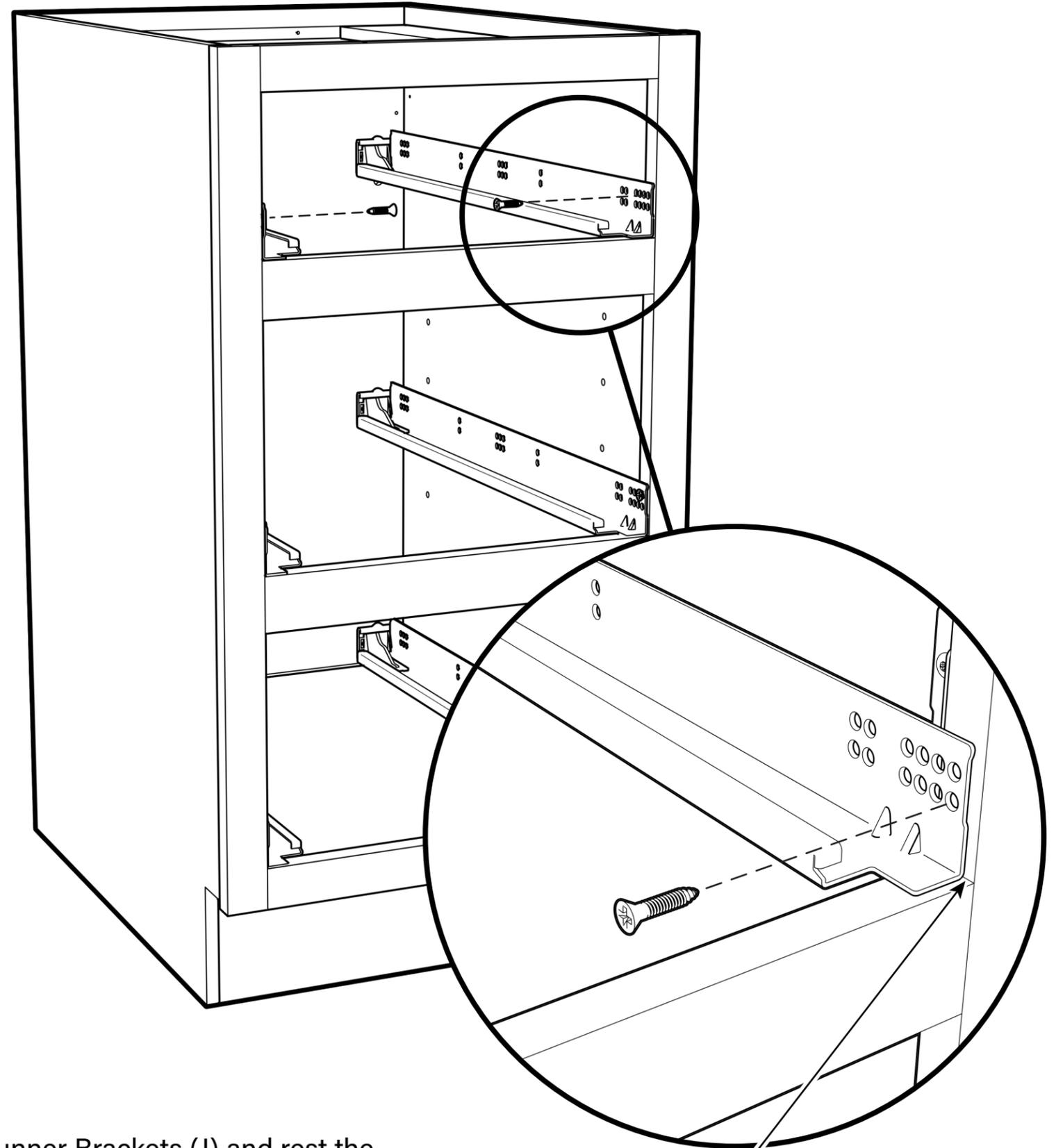
Runner should be set back slightly, so the screw is located in the center of the frame
