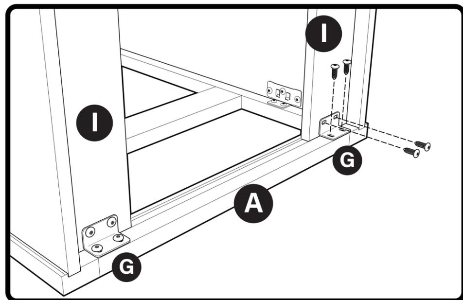
Secure the I-beams (I) to the back of the Frame (A) with (2) silver L-brackets (G) using (8) #8 x 1/2" Pan Head screws.
