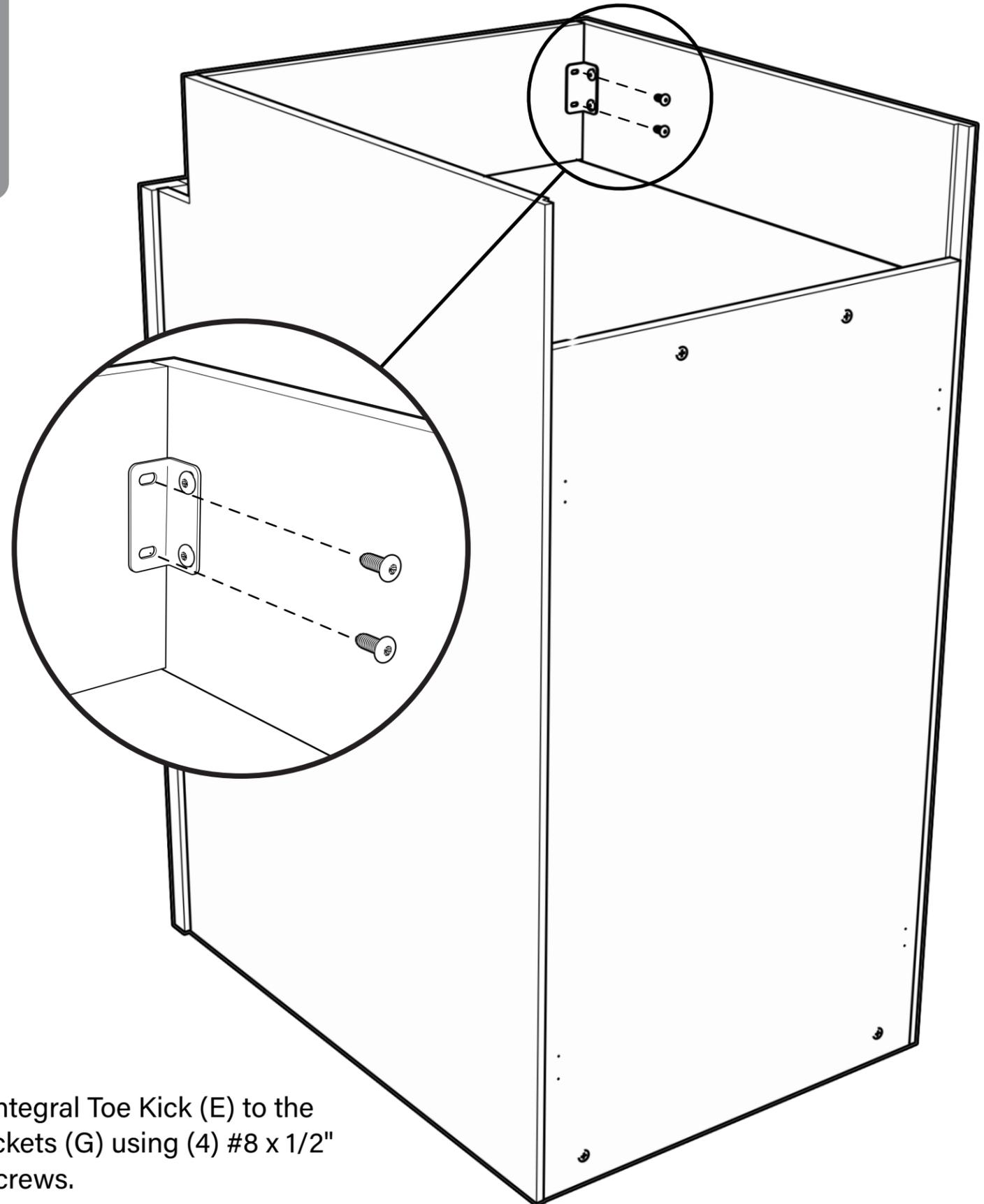
Mount the integral Toe Kick (E) to the silver L-brackets (G) using (4) #8 x 1/2" Pan Head screws.
