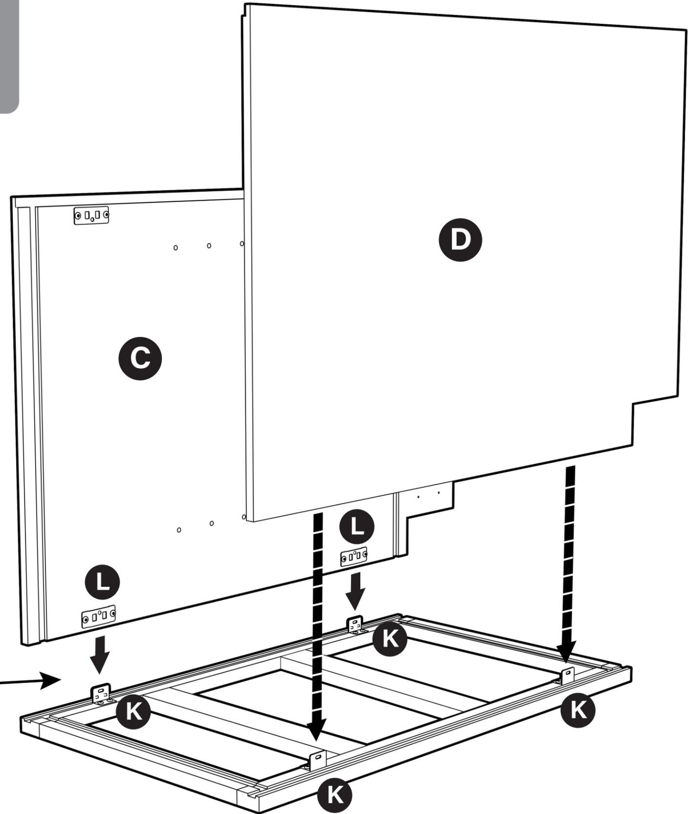
Run a bead of wood glue in the vertical grooves in the Frame (A) and insert End Panels (C and D), so that L-Brackets (K) & Connector Plates (L) snap together. Align the End Panels with the Frame, so that the dado grooves line up. Now, tighten all the Connector Plate screws and secure the Connector Plates and L-Brackets with (4) locking screws: #6 x 1/2" Pan Head.
