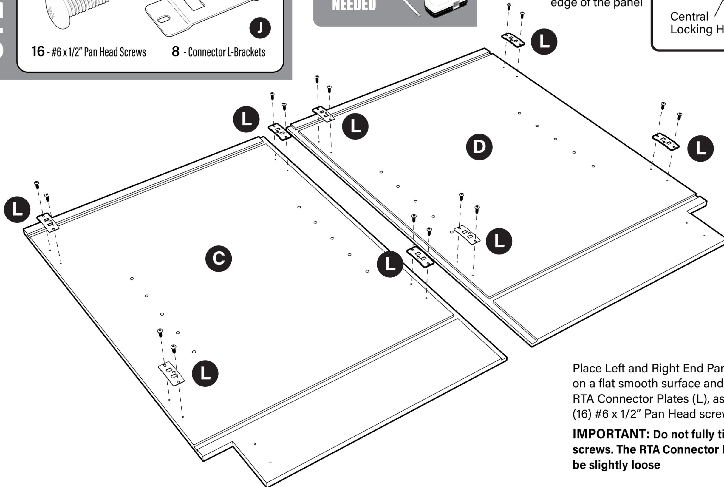
Place Left and Right End Panels (C and D) on a flat smooth surface and install (8) x tan RTA Connector Plates (L), as shown, using (16) #6 x 1/2" Pan Head screws.
