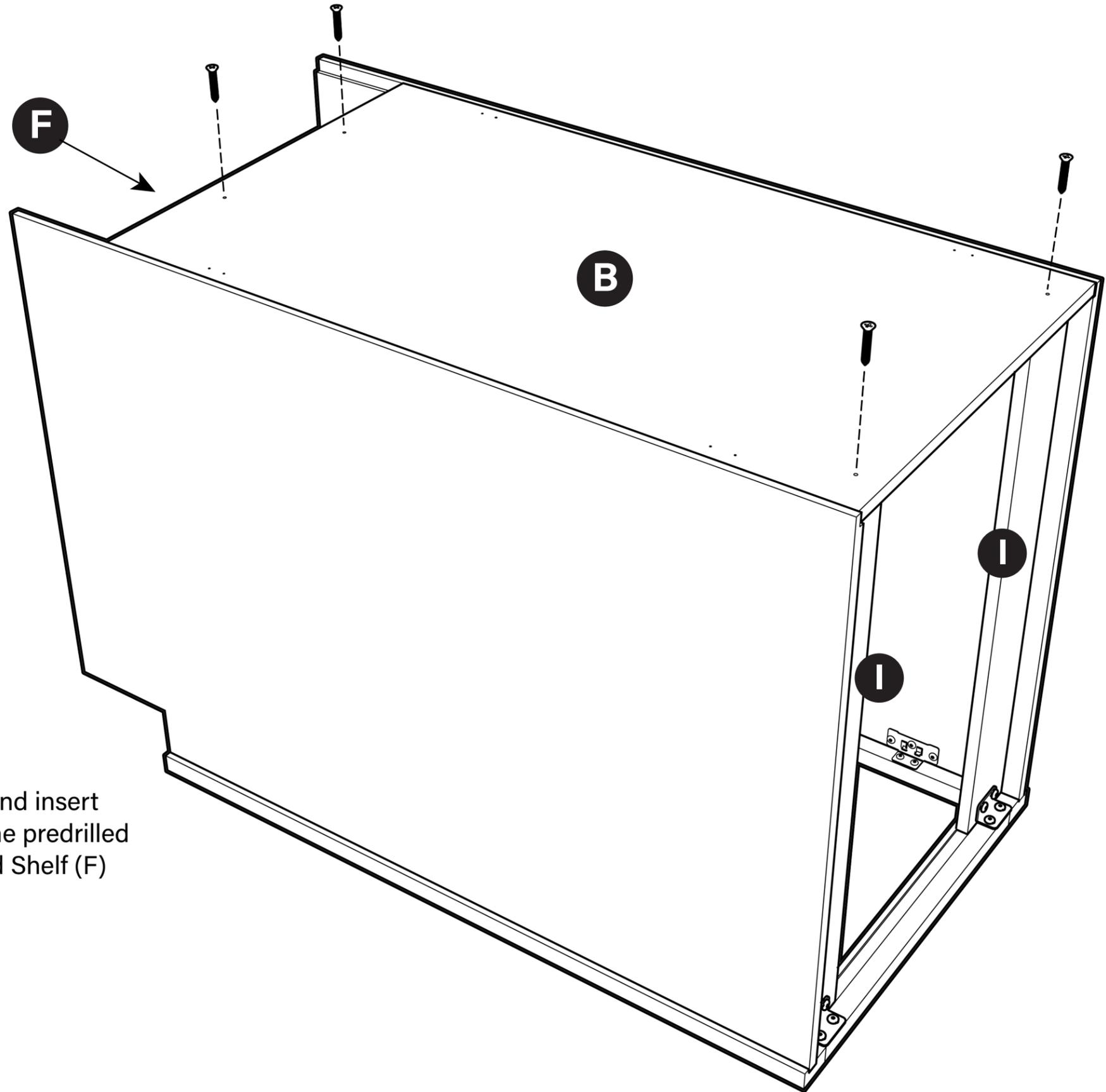
Make sure Back Panel (B) is correctly installed and insert (4) #6 x 1" Countersunk Flat Head screws thru the predrilled holes. Tighten the screws securely into the Fixed Shelf (F) and I-beams (I)."
