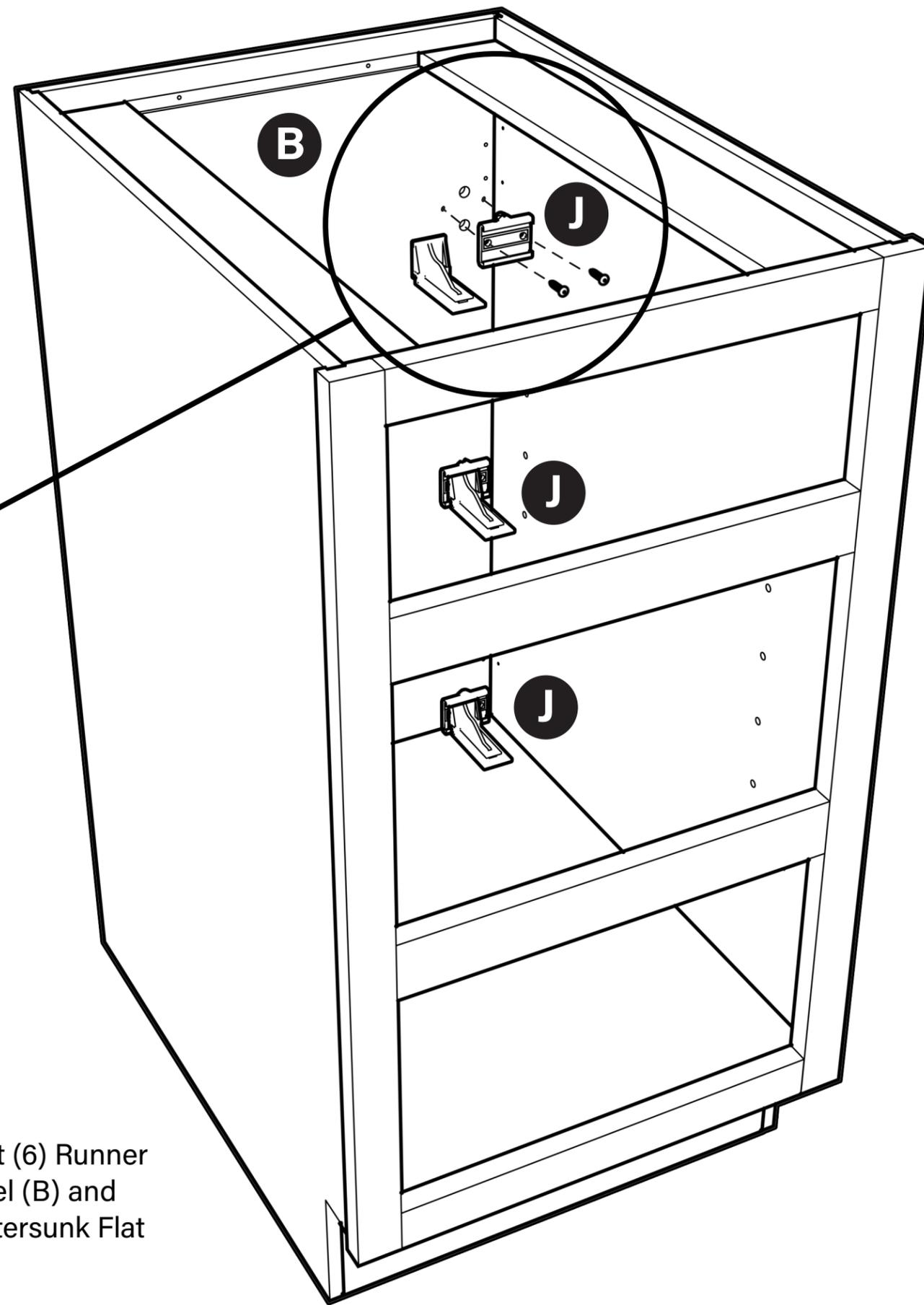
Stand cabinet upright and insert (6) Runner Rear Brackets (J) into Back Panel (B) and secure with (12) #6 x 5/8" Countersunk Flat Head screws.
