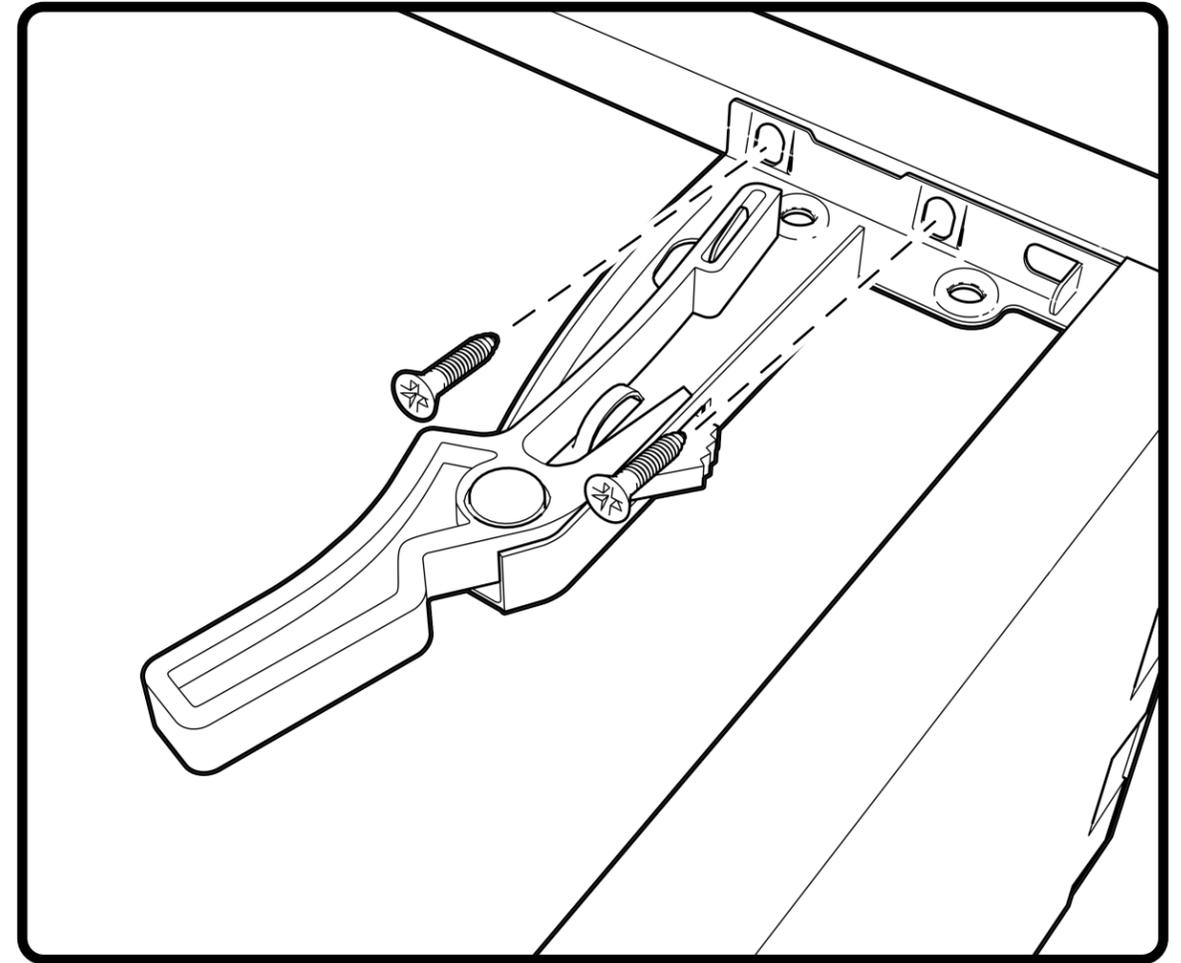
Turn drawers over and install (2) Locking Devices (V and W), to each drawer as shown, using (12) #6 x 5/8" Flat Head screws. Do not overtighten the screws
