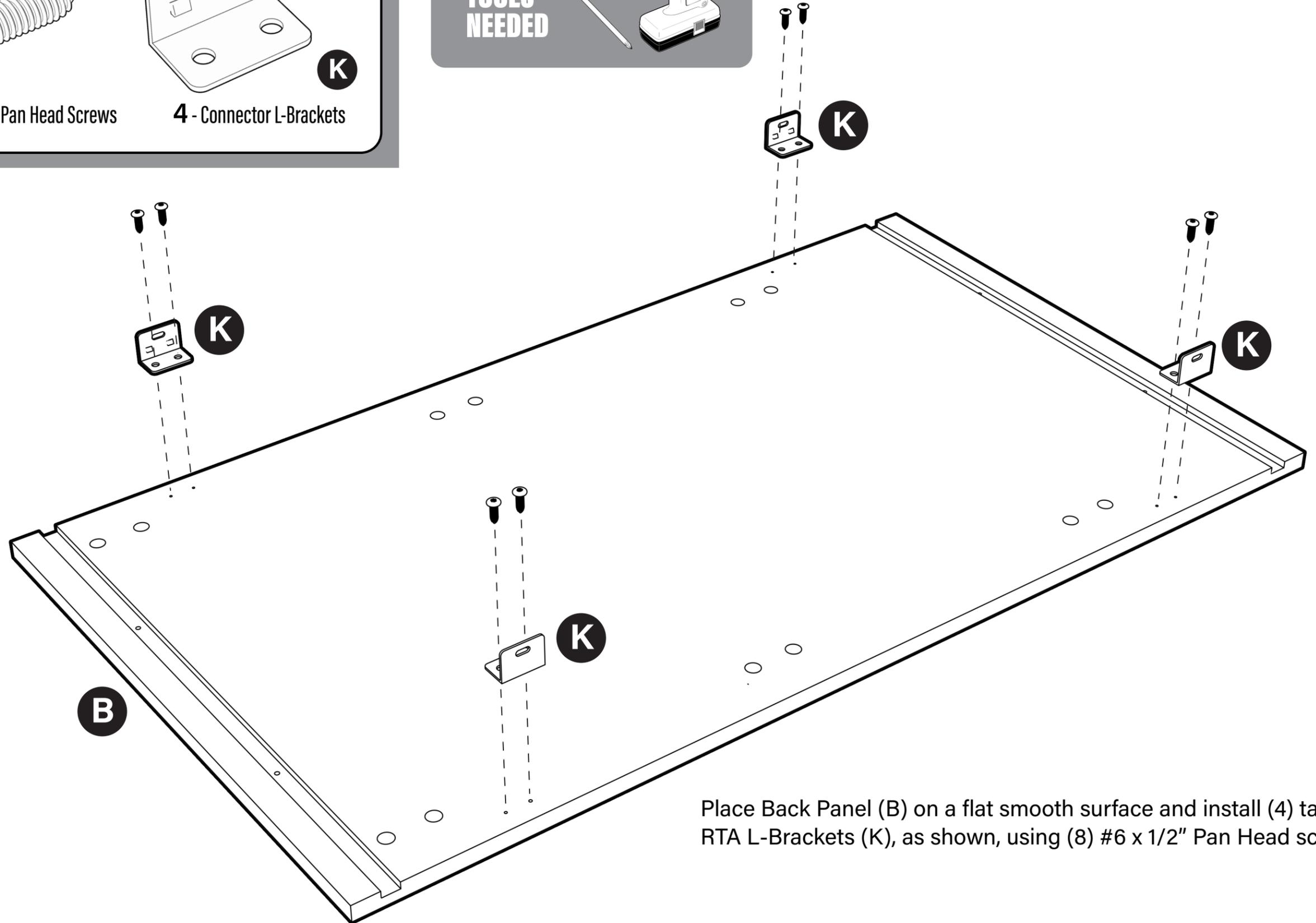
Place Back Panel (B) on a flat smooth surface and install (4) tan RTA L-Brackets (K), as shown, using (8) #6 x 1/2" Pan Head screws.
