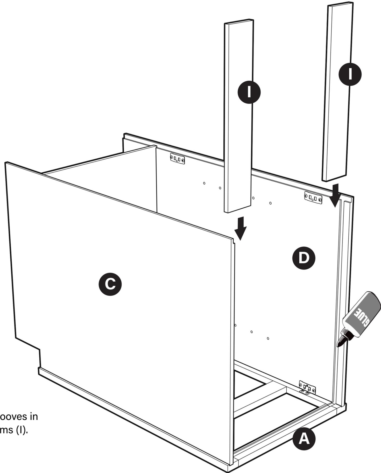
Run a bead of wood glue into upper horizontal grooves in the End Panels (C and D) and insert the (2) I-beams (I).
