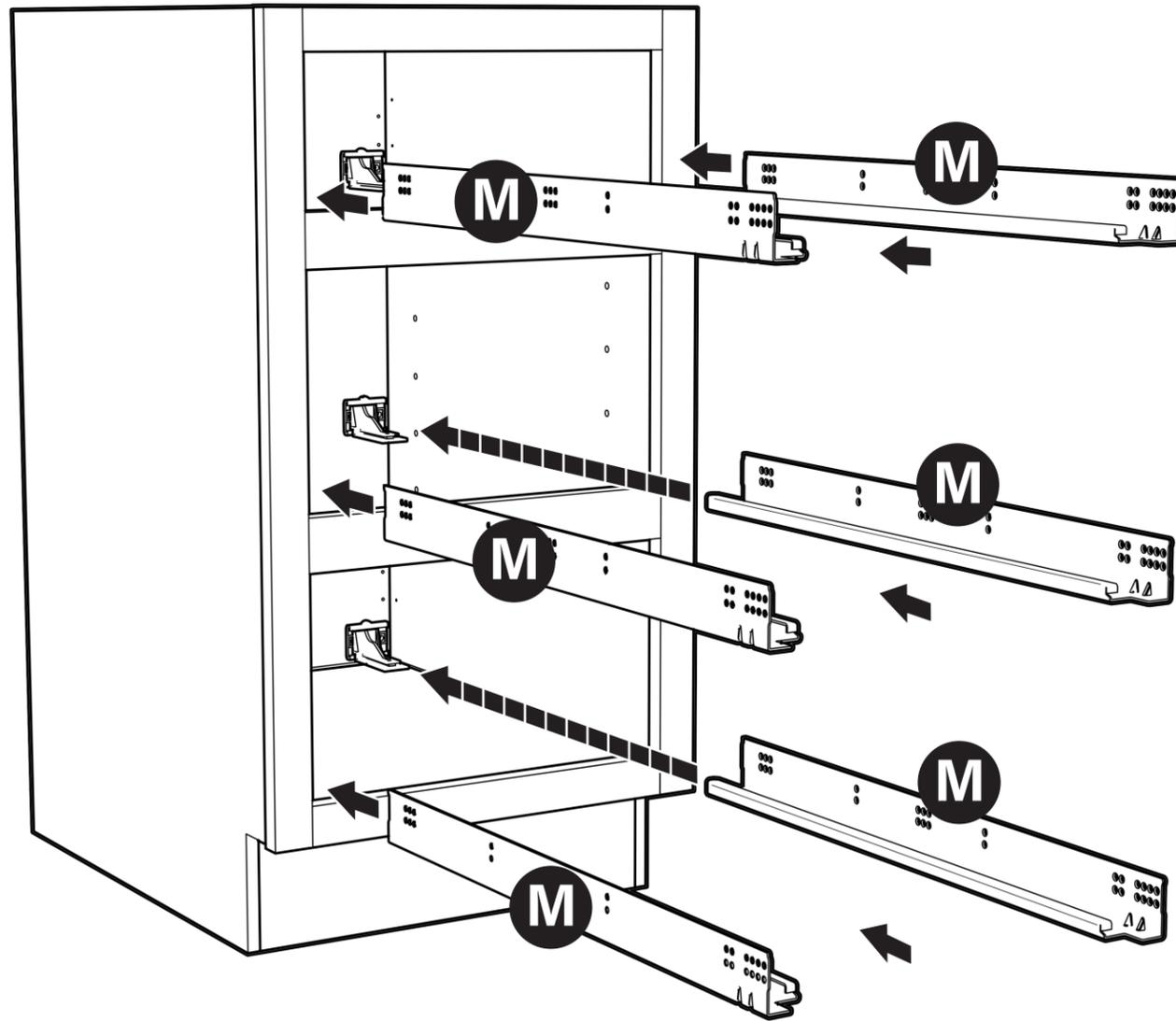
Slide Drawer Runners (M) into Runner Brackets (J) and rest the front of the runners on the Frame (A). Secure the runners to the side frame with (2) #6 x 5/8" Countersunk Pan Head screws.
