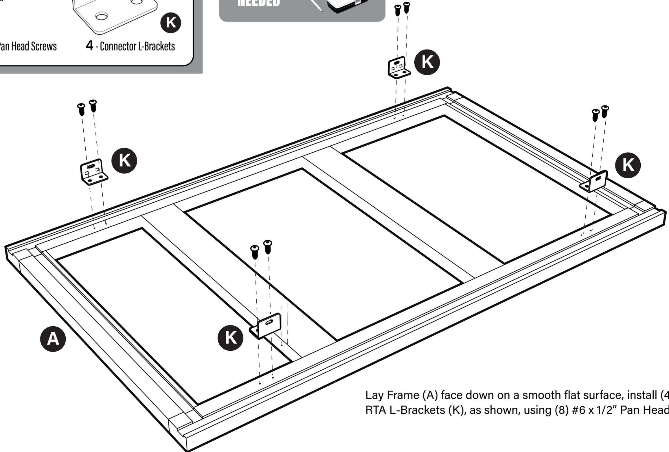
Lay Frame (A) face down on a smooth flat surface, install (4) tan RTA L-Brackets (K), as shown, using (8) #6 x 1/2" Pan Head screws.
