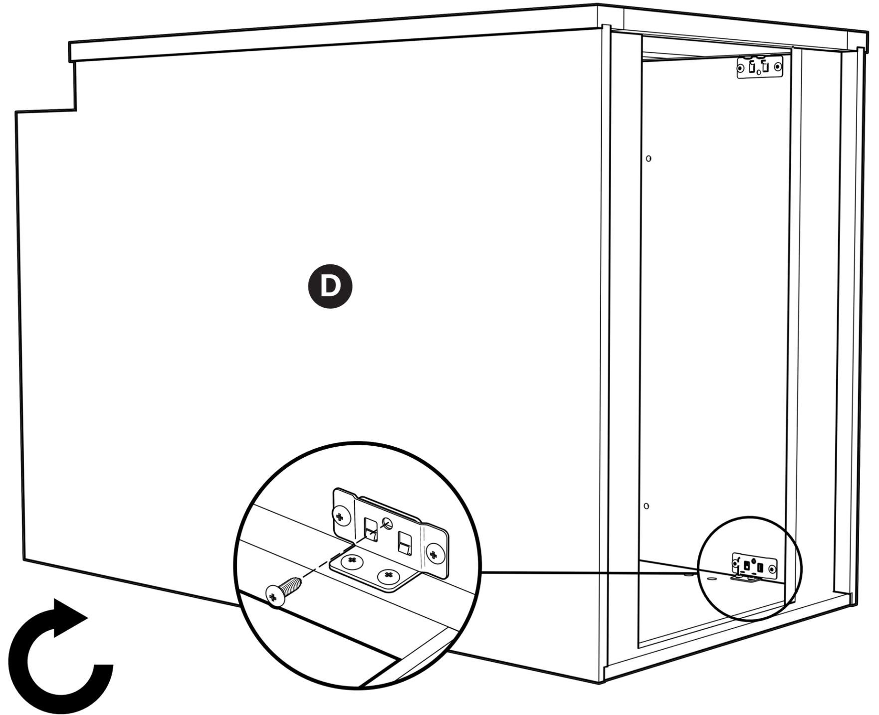
Carefully turn the cabinet over, make sure it is square, tighten all the Connector Plate screws and then secure the Connector Plates and L-Brackets with (4) locking screws: (4) #6 x 1/2" Pan Head screws.
