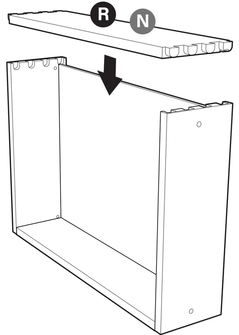
Slide the Drawer Bottom (U) into the grooves and install the other Drawer Side. If necessary, use a rubber mallet to gently tap the joints into place.
