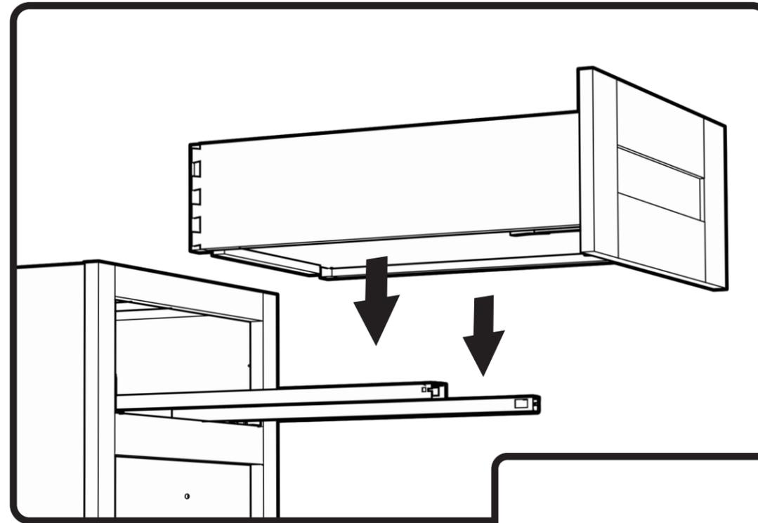
3 Under the drawer, slide the runners forward until they lock into the Locking Devices. Then close drawer to fully engage. The metal prongs on the back of the runner should be inserted in the holes in the back of the drawer
