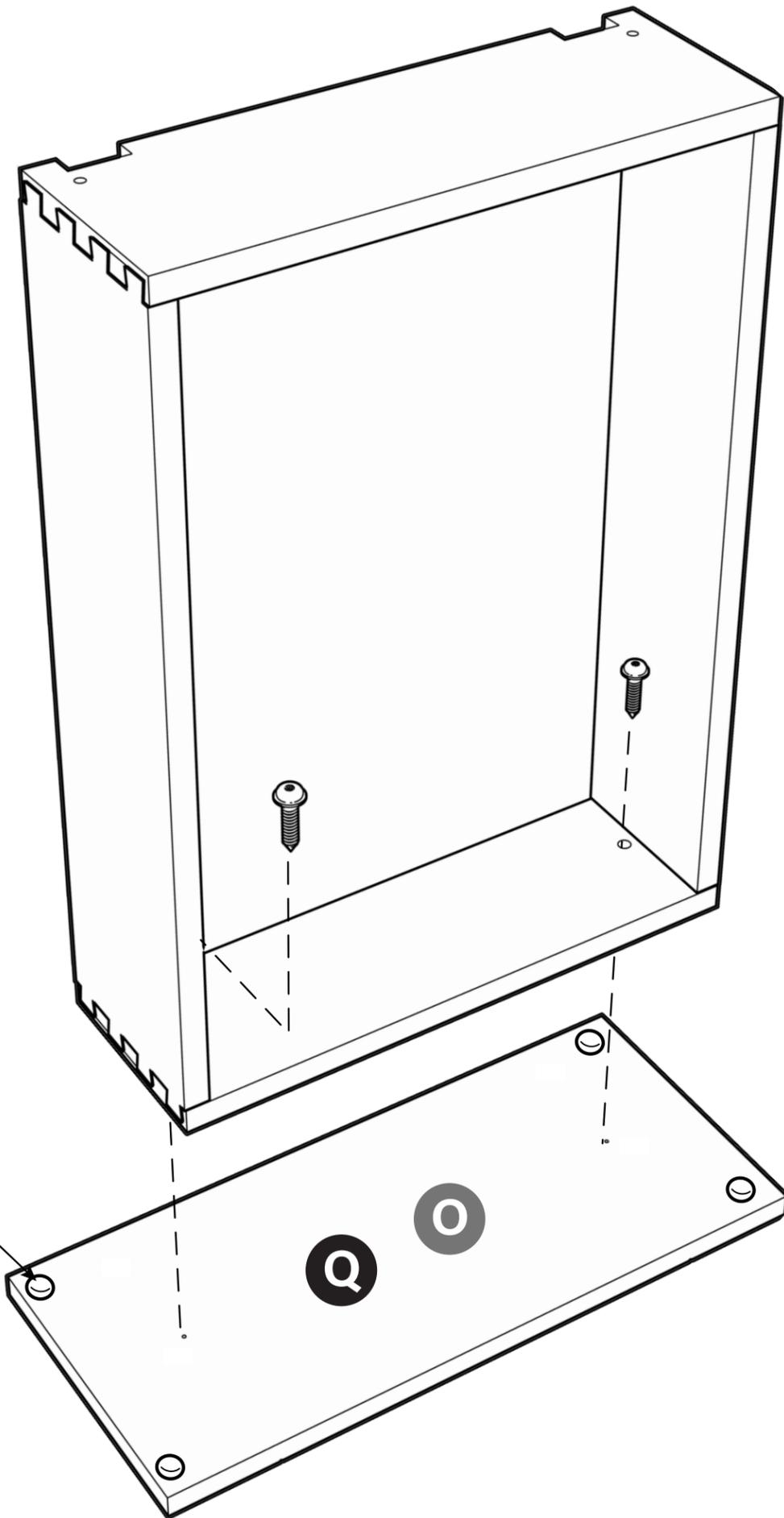
Lay the decorative Drawer Fronts (Q or O) face down on a smooth flat surface and install a clear bumper in each corner. If the (2) pilot holes in the back of the Drawer Fronts are barely visible, we recommend you enlarge them by partially inserting and then removing the attachment screws.
