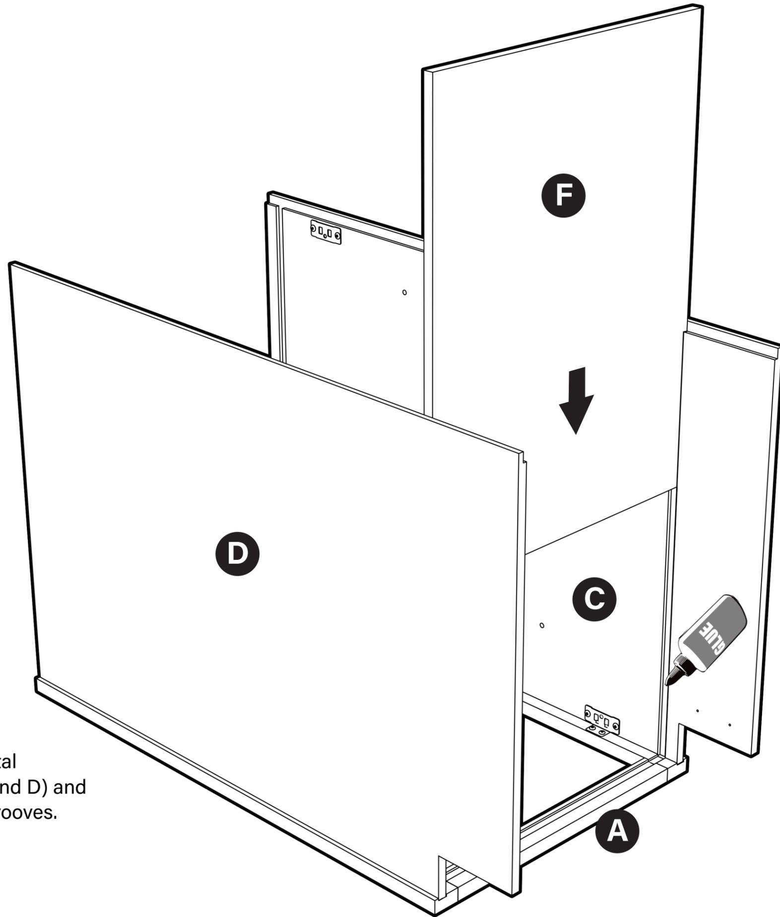
Run a bead of wood glue in the lower horizontal grooves in the Frame (A) and End Panels (C and D) and slide the Fixed Shelf (F) completely into the grooves.
