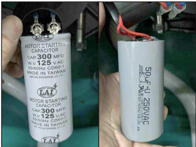
Figure 29. Start and run capacitors.
