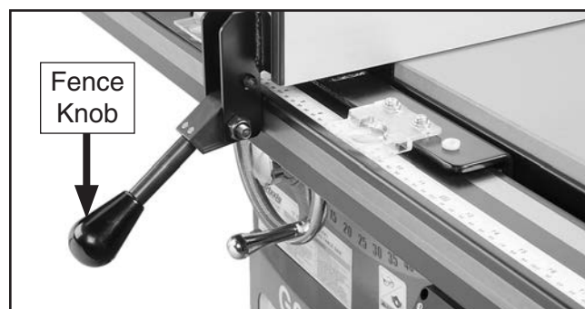
Figure 19. Fence knob installed.
