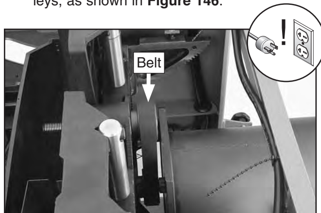
Figure 146. Belt installed (table removed for clarity.)
