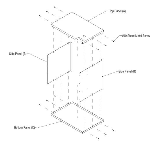
4. Position the assembled filter box on rear of furnace, supporting it firmly up to electrical enclosure covering the rear distribution blower. Make sure the filter box is tightly pressed to the back of the furnace. Use 6 #8 self-tapping screws (included) to firmly attach the filter box to alignment holes on sides of furnace.
