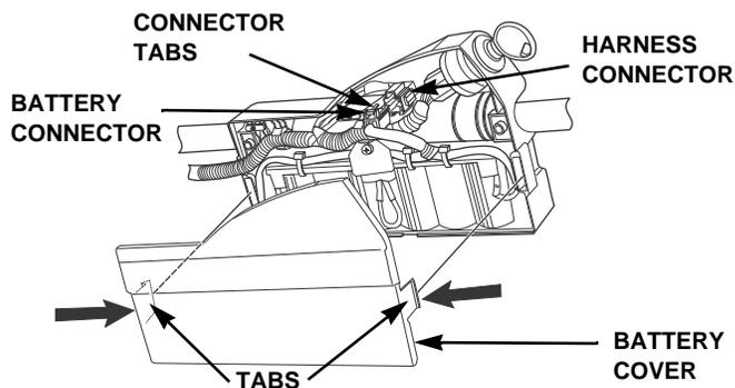
3. Connect the battery connector to the charger supplied with the mower.
