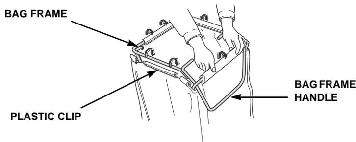
Lift the discharge guard and install the grass bag.
