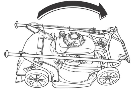
When unfolding the handlebar, be sure to lock the adjust knobs to secure the handlebar in the mowing position (see page 3).
