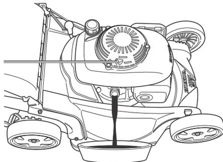
The used oil will drain through the filler neck. Allow the oil to drain completely.
