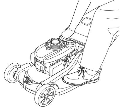
To ensure easy restarting and maximum performance from the Auto Choke System™, allow the engine to run for at least three minutes after starting a cold engine before shutting down. This minimum run time will be longer if the temperature is below 70°F (21°C).
