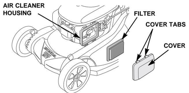
1. Press down on the cover tabs and remove the cover.
