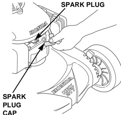
2. Remove the spark plug with a 13/16 in (21 mm) spark plug wrench.
