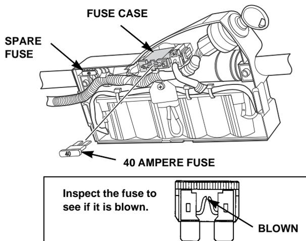
If a frequent fuse failure occurs, it usually indicates a short circuit or an overload in the electrical system. Take the mower to an authorized Honda servicing dealer for repair.
