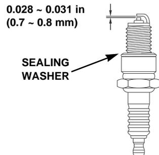
5. Install the spark plug carefully, by hand, to avoid cross-threading.
