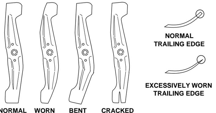
If a blade is bent, take the lawn mower to an authorized Honda servicing dealer for inspection.
