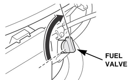
4. If your equipment will not be used for 3 to 4 weeks, we recommend running the engine's carburetor out of fuel. You can do this by leaving the fuel valve OFF, restarting the engine and running it out of fuel. See "Fuel" on [page 16](#) for periods of inactivity that exceed 4 weeks.
