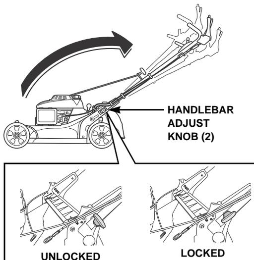
2. Align the adjust knobs with one of the three holes on the handle stay.
