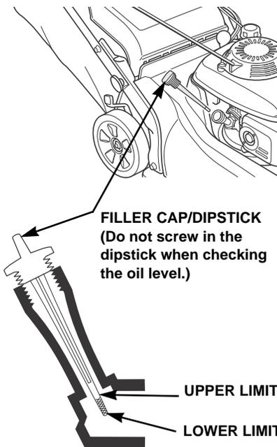
Do not overfill the engine with oil. If the engine is overfilled, the excess oil may get transferred to the air cleaner housing and air filter.
