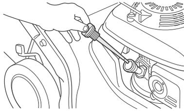
2. If the oil level is low, add oil to reach the upper limit mark on the dipstick. Do not overfill. If the engine is overfilled, the excess oil may get transferred to the air cleaner housing and air cleaner filter.
