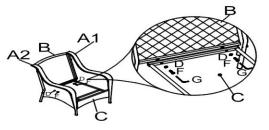
arms (A1.A2) with 4 washer (D) and 4 screws (F) by using allen wrech (G). Do not fully
