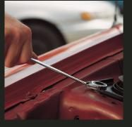
15° offset allows for safe operation above the work surface, providing additional knuckle clearance.
