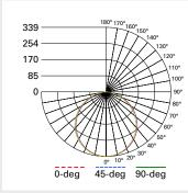
RLWZDZT56 (2700K) Spacing criterion (0/90/45): 1.26 / 1.26 / 1.38 Beam Angle: 112° Field Angle: 162° Lumens: 960 Input Watts: 9.4 W Efficacy: 102.1 LPW Test Report: RLWZDZT56-3000K.ies
