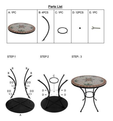
Step 1: Place the topper (A) on a leveled surface. Take one leg (B) and using 2 screws (D) assemble to table topper (A), tighten with wrench (E). Repeat this step with the other 3 legs (B), as shown on diagram above.
