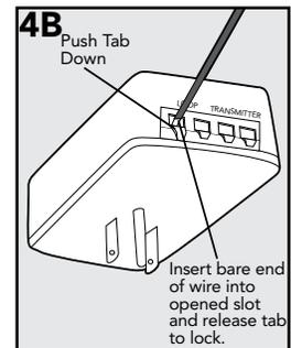
5. Determine the length of wire needed to pass from the Surge Protector to the Fence Transmitter. Measure and cut 2 lengths of wire, then strip  $\frac{3}{8}$  inch of insulation at both ends. Twist the 2 lengths together, with at least 10-12 twists per foot, so the wires will not send out a signal.
