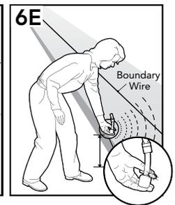
7. Test in a number of different locations around the containment area until you are satisfied that the system is functioning properly.
