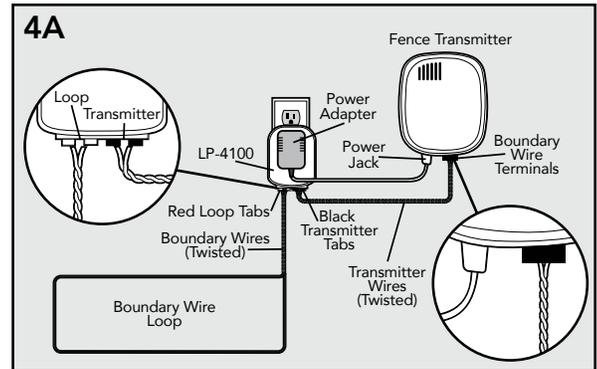
4. Strip  $\frac{3}{8}$  inch of insulation from the ends of the Boundary Wire. Insert the stripped ends into the 2 left red connector holes on the bottom of the Surge Protector labeled "Loop" (4B). There should be 1 wire in each connector hole. Press the plastic tab, insert the wires and release the tab. Make sure the wires do not touch each other at the terminals.
