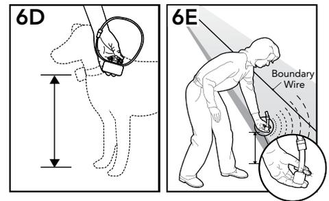
7. Test in a number of different locations around the containment area until you are satisfied that the system is functioning properly.
