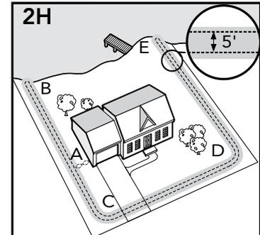
**Sample 5 (2H): Lake Access (Double Loop)** From the Fence Transmitter, run the wire to **A**, **A** to **B**, make a U-turn and go to **C**, **C** to **D**, **D** to **E**, make a U-turn and follow your path all the way back to **A** keeping wire separated **at least 5 feet**. Twist the wire from **A** back to the Fence Transmitter.
