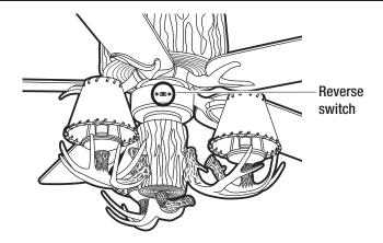
Cool weather - (Clockwise Direction) An upward air flow moves warm air off the ceiling. This allows you to set your heating unit on a cooler setting without affecting your comfort.
