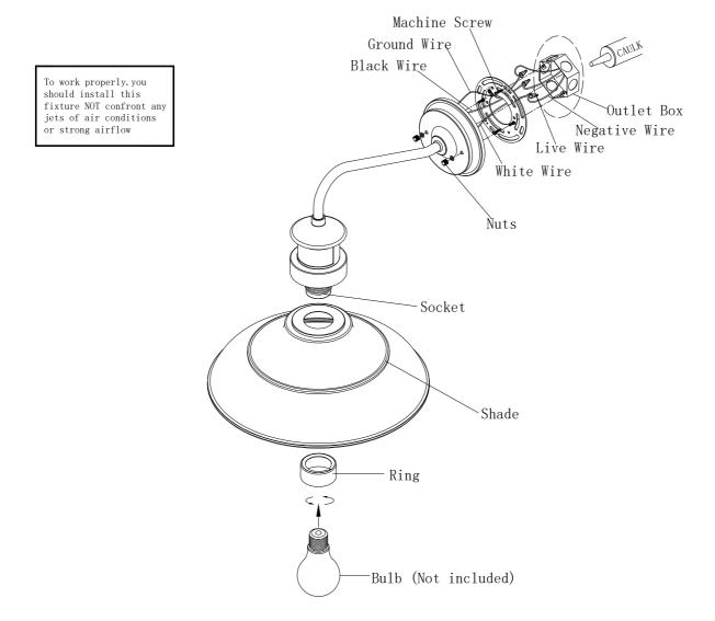
2. Pull out the wires and grounding wire from the outlet box. Make wire connections using the wire nuts, as follow: ---Connect the hot wire(usually black insulation) from the fixture to the black wire from the power source.
