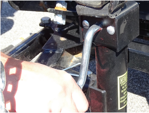
3. Adjust crankstand until until it is no longer in contact with the ground.
