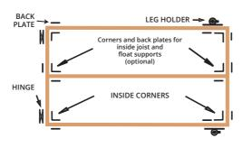
Arrange the float supports (2" x 6" boards) and floats on the structure to determine their positions. Leave +/- 6" of spacing with the main structure to allow further manipulations . Mark the locations of the float brackets on the structure and those of the floats on the supports. Remove the floats, bolt the float supports with brackets and secure the floats using lag screws and large flat washers. You can also use bolts with lock and flat washers.
