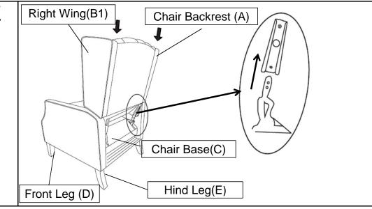
With assistance from your adult partner, hold up the fully assembled Chair Backrest (A) with Right Wings(B1) and Left Wing(B2), stand behind the chair. Insert the small metal arms on the sides of the Chair Backrest(A) into the prefabricated slide lock gadget on the Chair Base(C) as shown above. Firmly but gently, push the Chair Backrest (A) downwards until the Chair Backrest(A) is fully slotted and locked into position.
