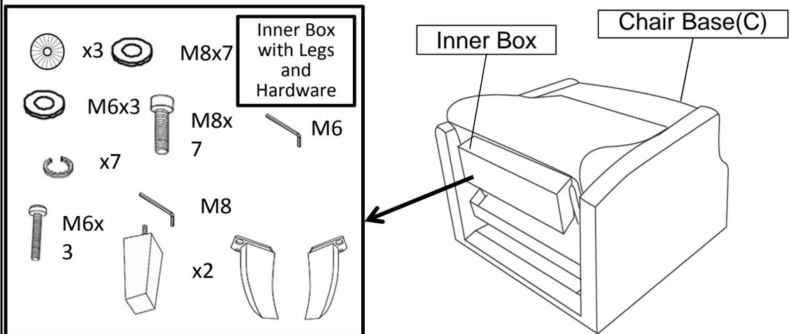
Place the Chair Base(C) on a clean, non-marring surface. Take out the four wooden legs and Hardware from inner box, as picture shown on above.
