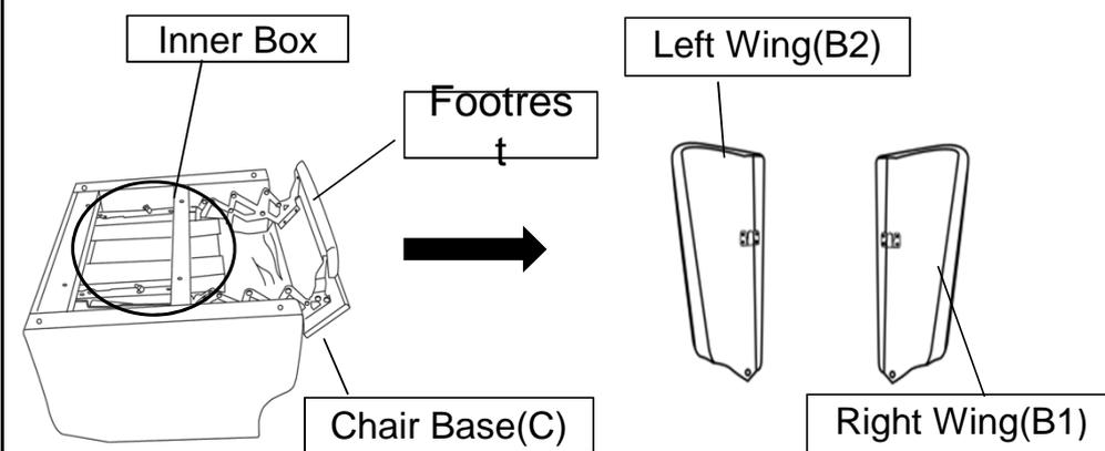
Turn the Chair Base(C) upside down on a clean, non-marring surface. Extend the Footrest to open. Carefully take out inner box stowed as shown above. Open it, and you will find Right Wings (B1) & Left Wing (B2). Stow the Footrest to original position.
