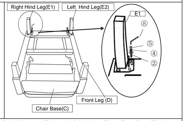
Attach the Right Hind Leg(E1) and Left Hind Leg(E2)to Chair Base(C) with Bolt(⑤), Washer Ring (④), Washer(②) with Allen Key(⑧) by turning the legs clockwise as shown.
