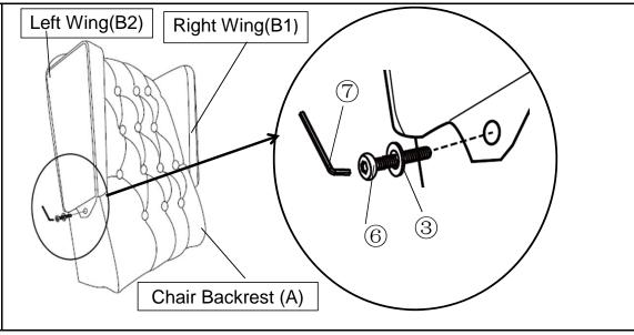
Attach Left Wing(B2) to the Chair Backrest(A) using Bolts(6) and Washer(3) with Allen Key(7). As picture shown .
