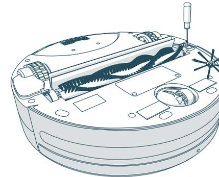
1. Remove the screw on the main brush using a flat head screwdriver.
