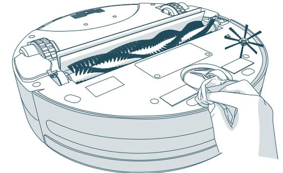
1. Wipe the obstacle/wall and edge sensors with a soft cloth slightly dampened with cold water or alcohol.
