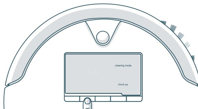
Press the **CLEANING MODE** button on Bob's cover. The main and side brushes should spin, and air should flow out of the dustbin.
