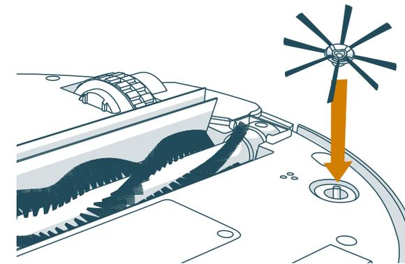
1. Flip Bob over onto a flat surface. Place the side brush over the empty socket on Bob's underside.
