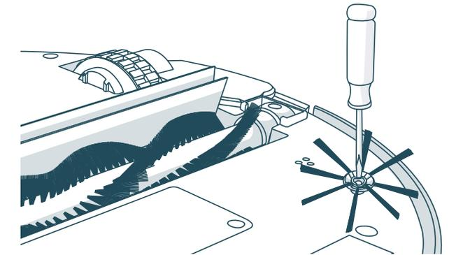
2. Secure Bob's side brush into the socket using the flat head screwdriver and screw.
