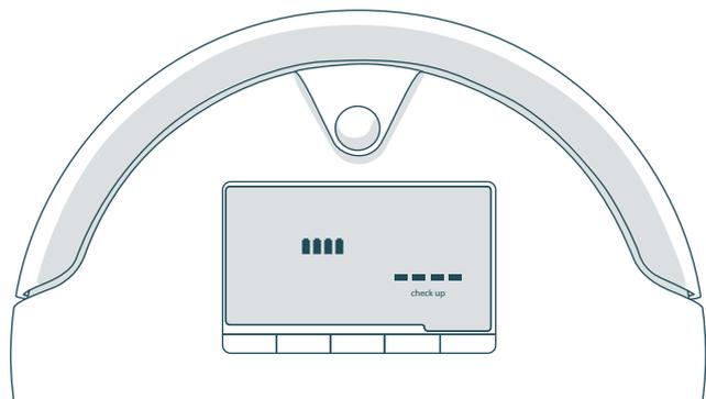
The 4 bars above the word “checkup” should be lit. Lift Bob about 6 inches (15 cm) off the ground and the 4 bars should turn off.
