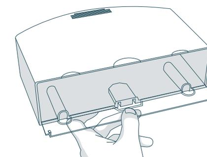
2. Carefully open the plastic gate and dump out the contents of the dustbin.
