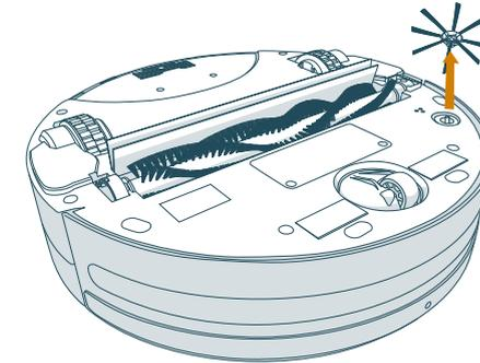
1. Remove the screw on the side brush using a flat head screwdriver.
