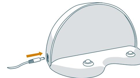
1. Plug the charging adapter into the side of the charging station. The station's red power light will turn on.
