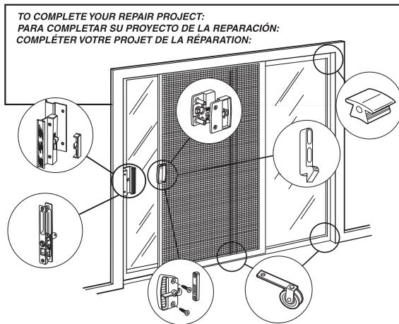
**INSTALLATION HINTS:** Remove inside and outside handle assemblies. Insert screwdriver into bottom mounting holes to prevent latch from dropping. Remove screws on lock face and angle latch out of door frame. Install new one in same manner. Re-install handles and check for smooth operation.
