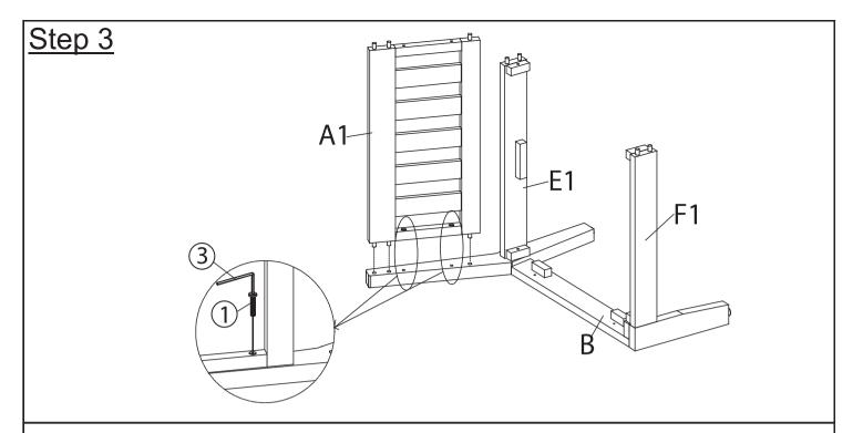
Insert dowels on Backrest Panel(A1) into mountings on Left Panel(B). Attach Left Panel(B) to Backrest Panel(A1) using Bolts(1) with Allen Key(3). Do not fully tighten the Bolts.
