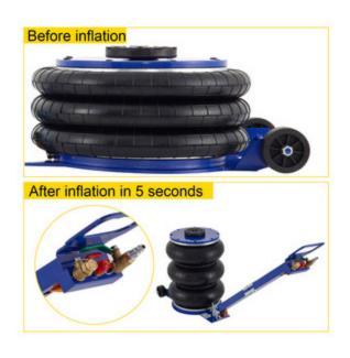
There are three valves on this triple airbag jack: air input valve, air outlet valve, safety valve, which can help you operate the jack
