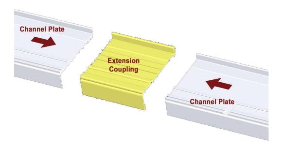
Use PVC Cement to attach. Extension coupling should be engaged a minimum of 2" on each side.
