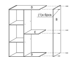
Attach Right Side Panel (B) to assembled unit
