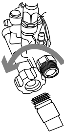
Figure 2-9. Connect Water Supply Hose
