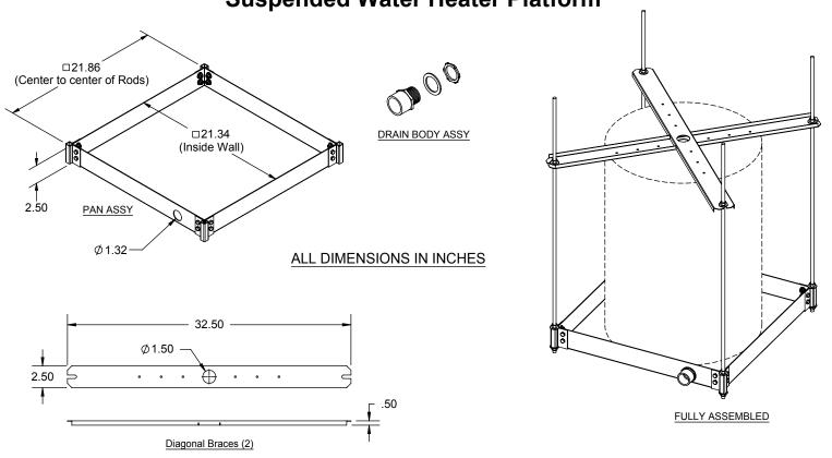
The Suspended Water Heater Platform is engineered to support water heaters up to 20 U.S. gallons (up to 375 pounds total weight). This time and labor savings tool is designed for the Professional Contractor. Design features requested by plumbers are incorporated into a professional platform that can be suspended with all thread rod.
