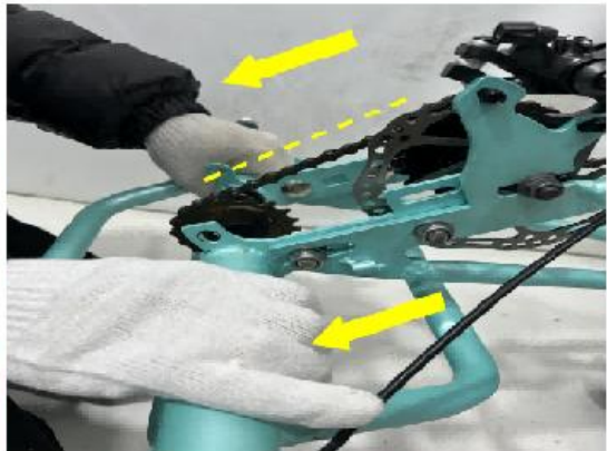
Pull the tripod back so the chain is taut and straight
