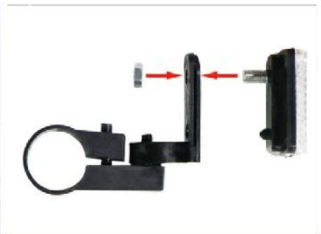
Assemble the front reflector
