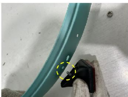
Insert the rear reflector screw into the hole as shown
