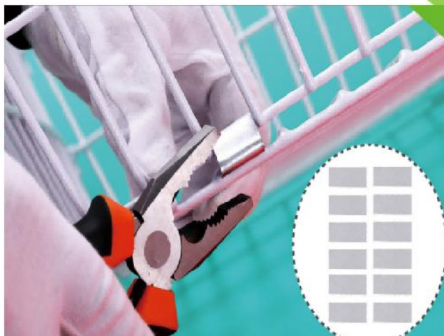
Secure with metal sheets
