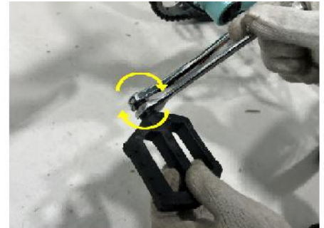
Grip the pedal and tighten it
