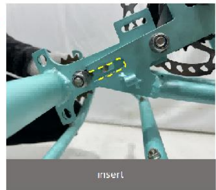
Note the combination of screws and nuts at the four positions in the
