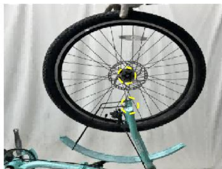
Assemble front wheel as shown
