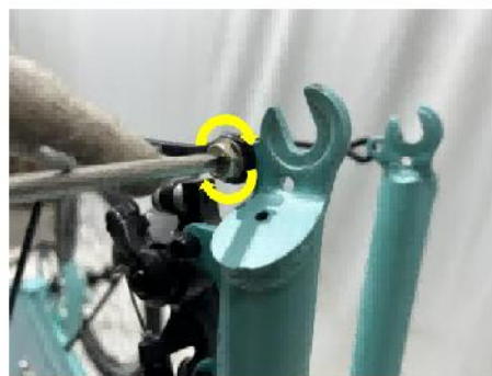
Lock both fender support rods in turn
