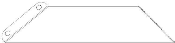
D06 CORBEL - A4M01832 (x1) 2 3/4"x5 7/8"x24 13/16" (70x149x631)
