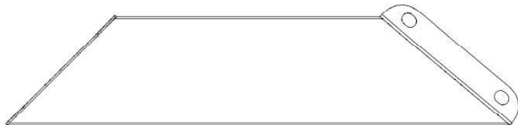
D05 CORBEL - A4M01831 (x1) 2 3/4"x5 7/8"x24 13/16" (70x149x631)
