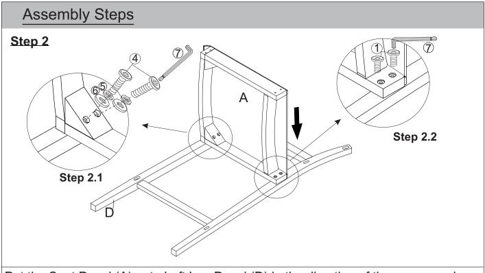
Put the Seat Panel (A) onto Left Leg Panel (D) in the direction of the arrow as shown in above picture.
