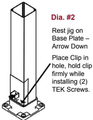
**STEP TWO - Securing Posts to Deck**
