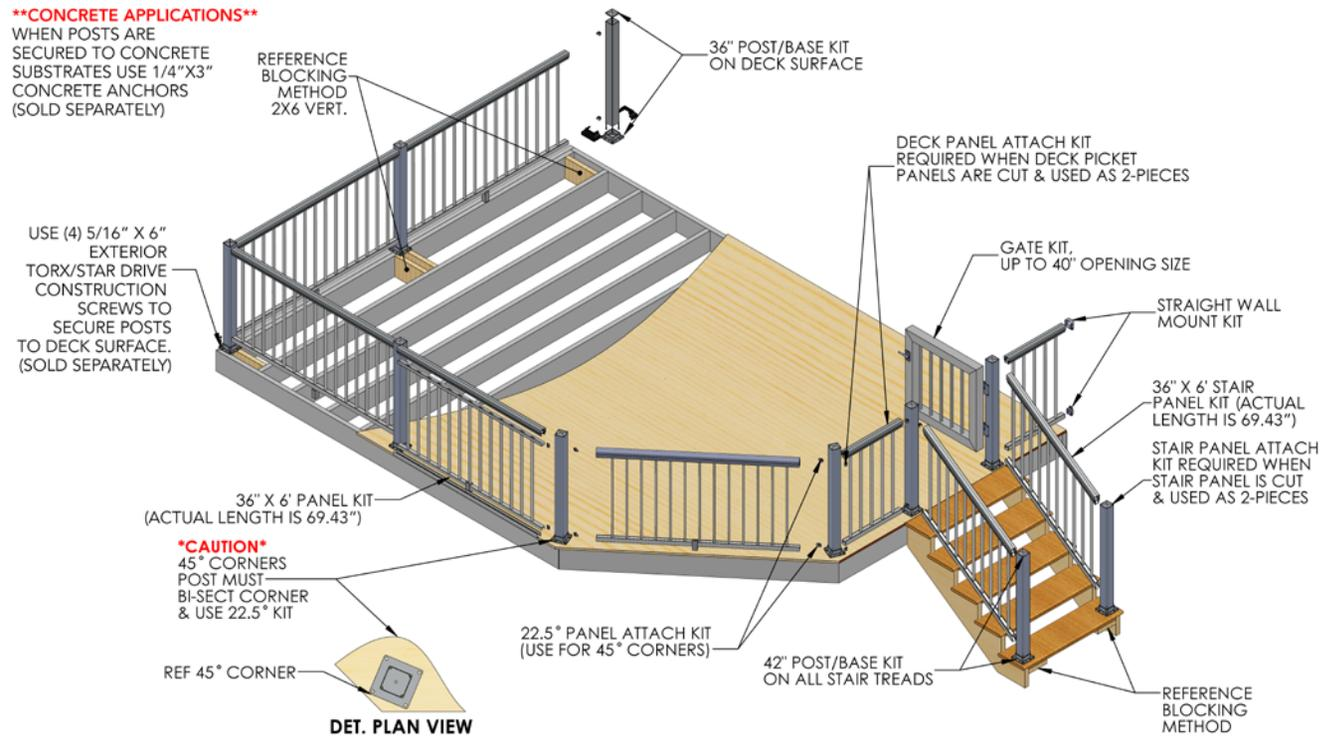
**STEP ONE – Determine necessary posts required and prepare (end, center or corner)**
