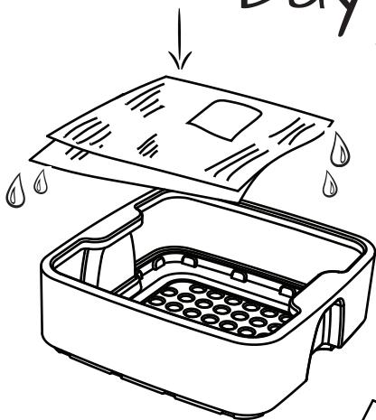
1. Set working tray on base, soak 2 sheets of newsprint in water, lay in bottom of tray. (initial setup only)
