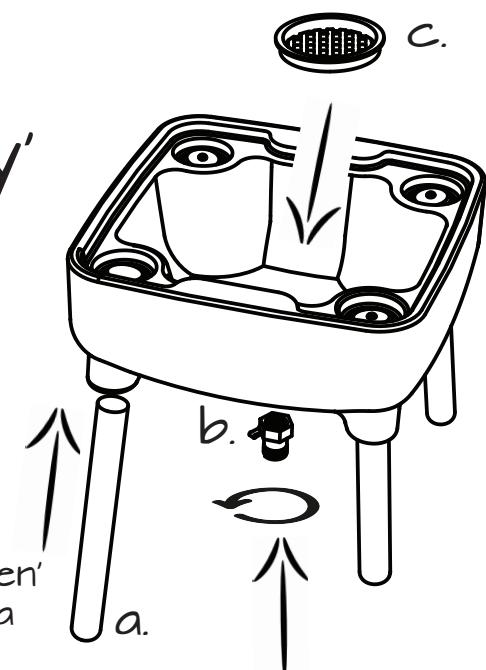
b. screw on 'drain valve' into the bottom of base
