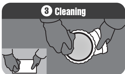
3 Cleaning Using a soft cloth wipe clean inside and outside of both pipe and compression fitting.
